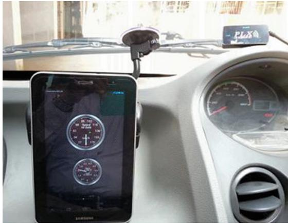
**Fig. 5** Experimental set-up displaying Bluetooth OBDII device and Tab as data logger
