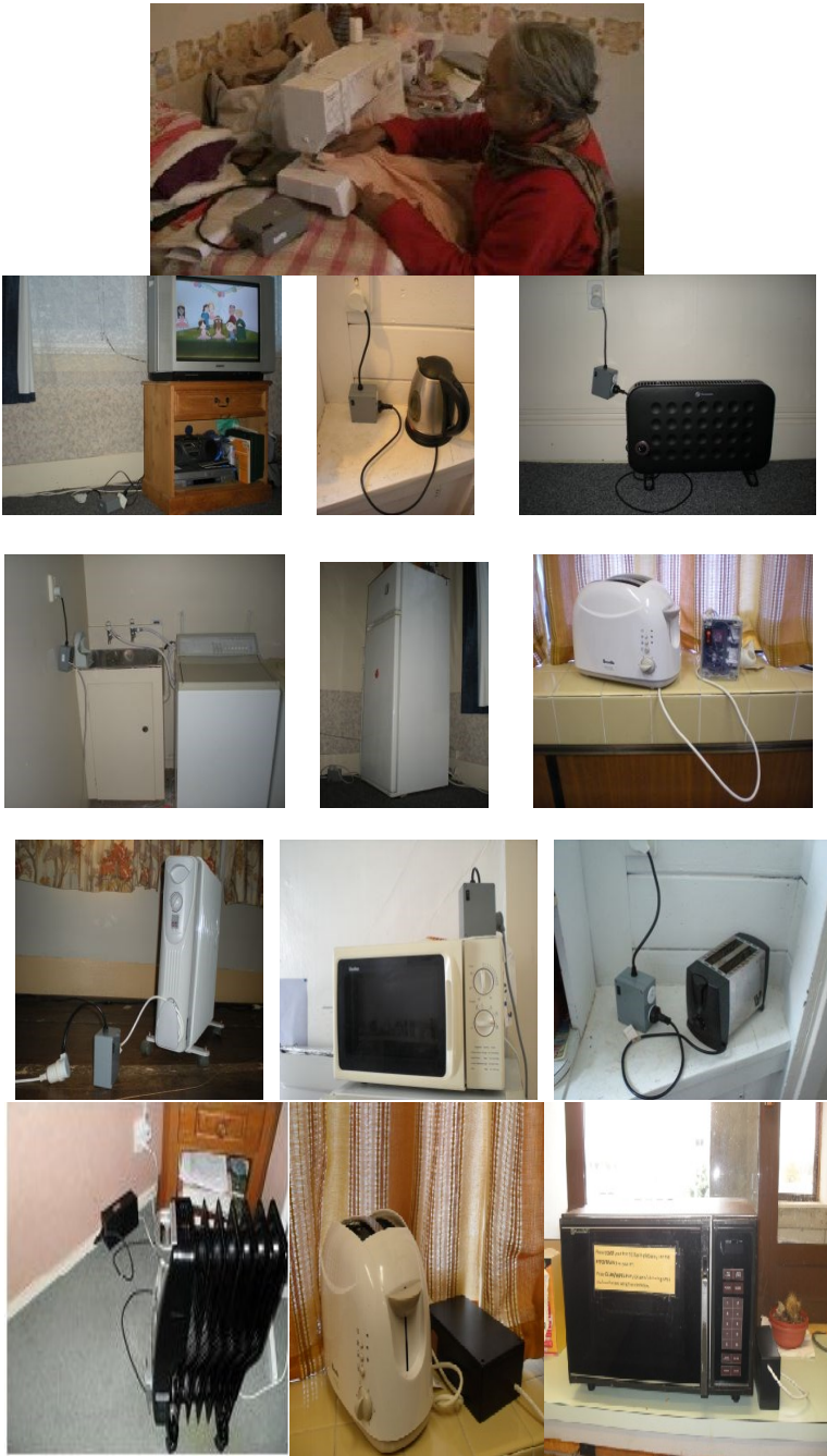
Fig. 3.7 Fabricated Wireless Electrical Sensing Systems attached to various Household Appliances
