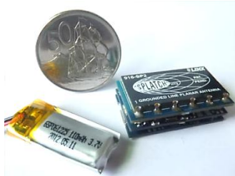
Fig. 1. AWSAM-3 featuring antenna, core, and power, beside a Li-Po battery and NZ50c coin
