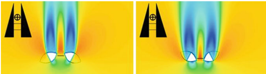
Fig. 4 Flow visualisation using CFD modelling-Bahrain world trade centre [5]
