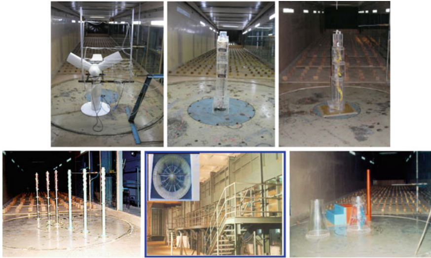
Fig. 2 Application of boundary layer wind tunnel testing on civil engineering industrial structures [3]
