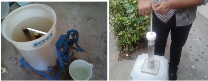
Fig. 8 Energy conservation through hand operated ultrafiltration for clarification and disinfection of flood water
