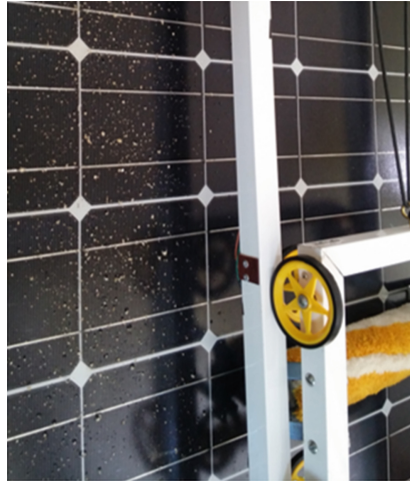
Fig. 7. Operation of the prototype showing the cleaned right section of the PV panel after one pass of Structure 2 while the left section remains dirty.
