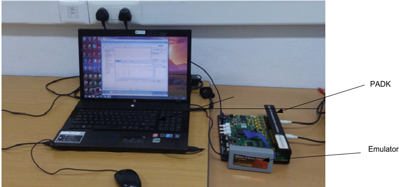
Fig. 1. Professional Audio Development Kit with the Blackhawk Emulator USB 560v2
