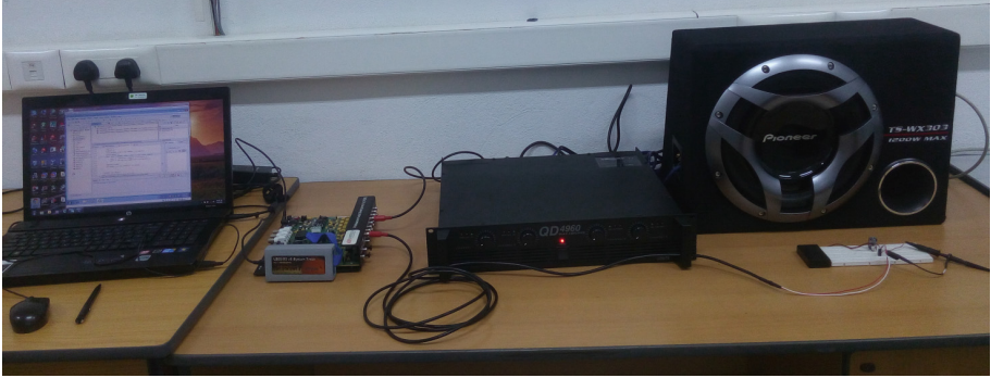
Fig. 4. System identification setup in acoustic domain.
