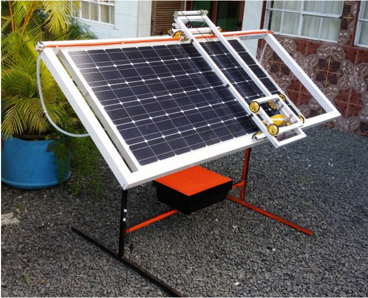
Fig. 6. Prototype of the low-cost autonomous PV array cleaner.
