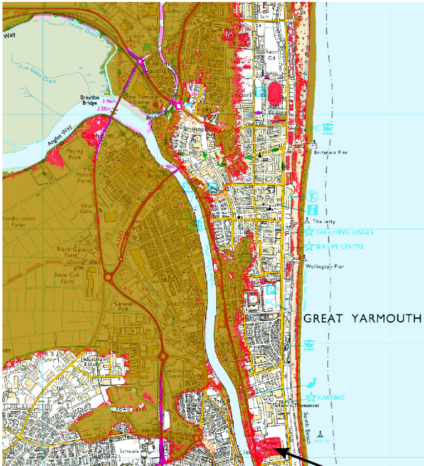
Figure 20.15. Potential inundation (without defences or in the event of a breach) for one of the most affected areas on 9 November 2007. The brown shading indicates the flood extent with sea levels of 2.86 m above ODN (as occurred); red areas are the additional inundation with sea levels of 3.24 m above ODN as predicted by the most extreme ensemble member. The black arrow (bottom right) shows the location of a power station.
