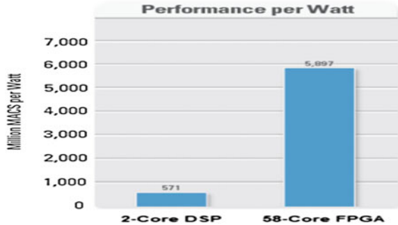
Fig. 1 Performance comparison (FPGA vs. conventional DSP processor). + MACS—Multiply–accumulate operations per second (measure of DSP performance)
