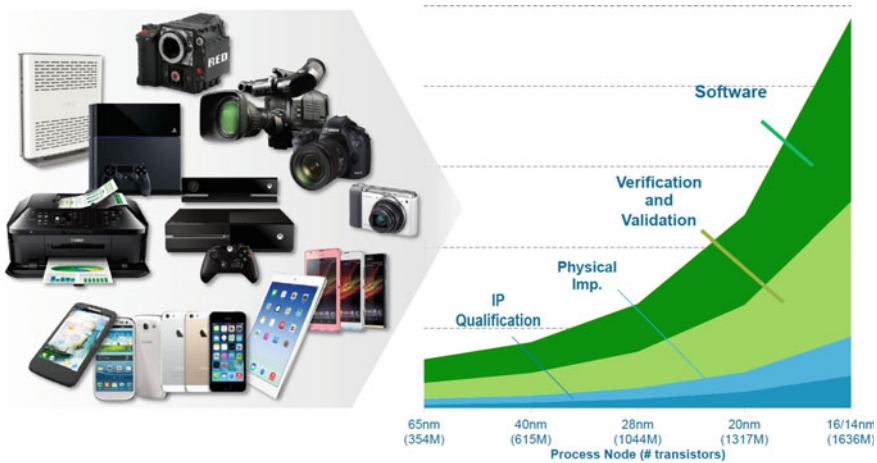
Fig. 1.3 Software and verification driving SoC project costs [37]
