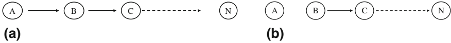
Fig. 5.8 a Synchronization after an event and b message forwarding for synchronization after an event
