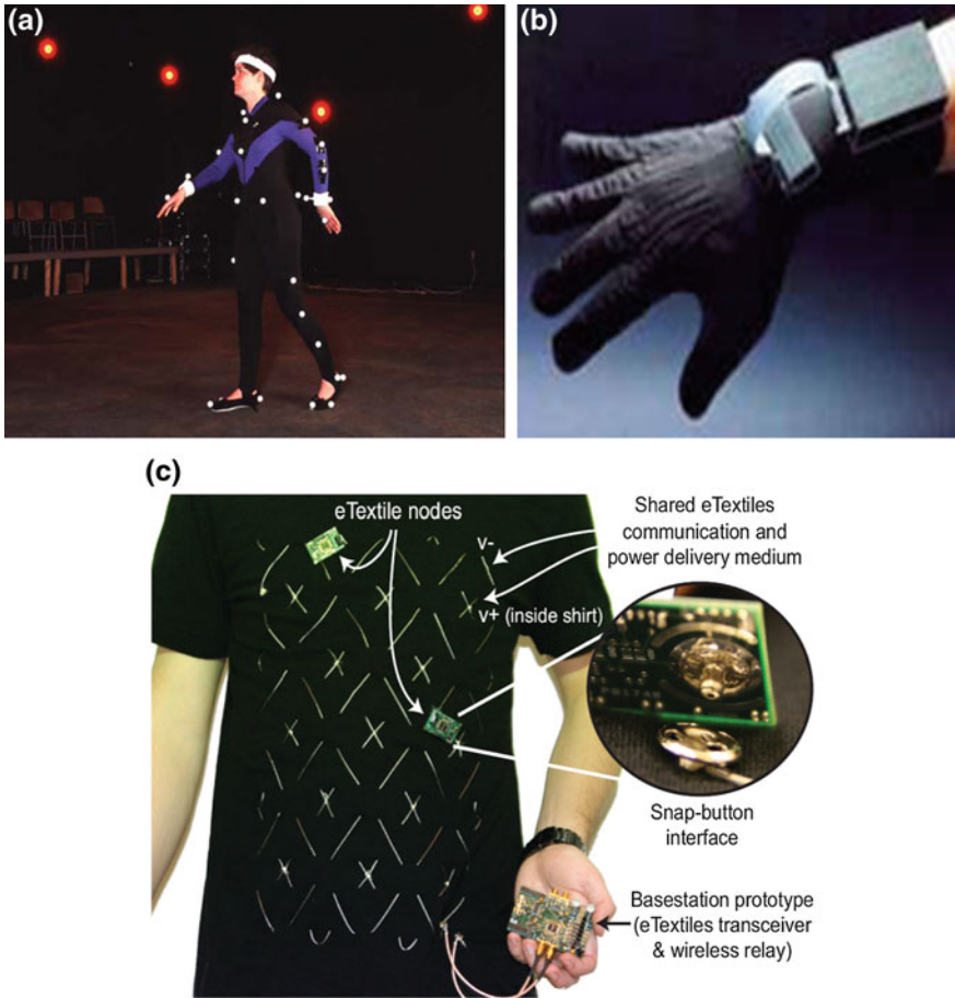
Fig. 16.12 a Reflective Markers b Fiber optic sensors c e-Textile SNs
