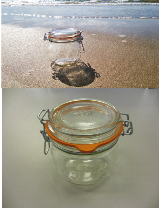
Fig. 2 Photograph of the sealed bottle for long-term LIBS in-situ measurement to detect the increased ratio of disintegration materials
