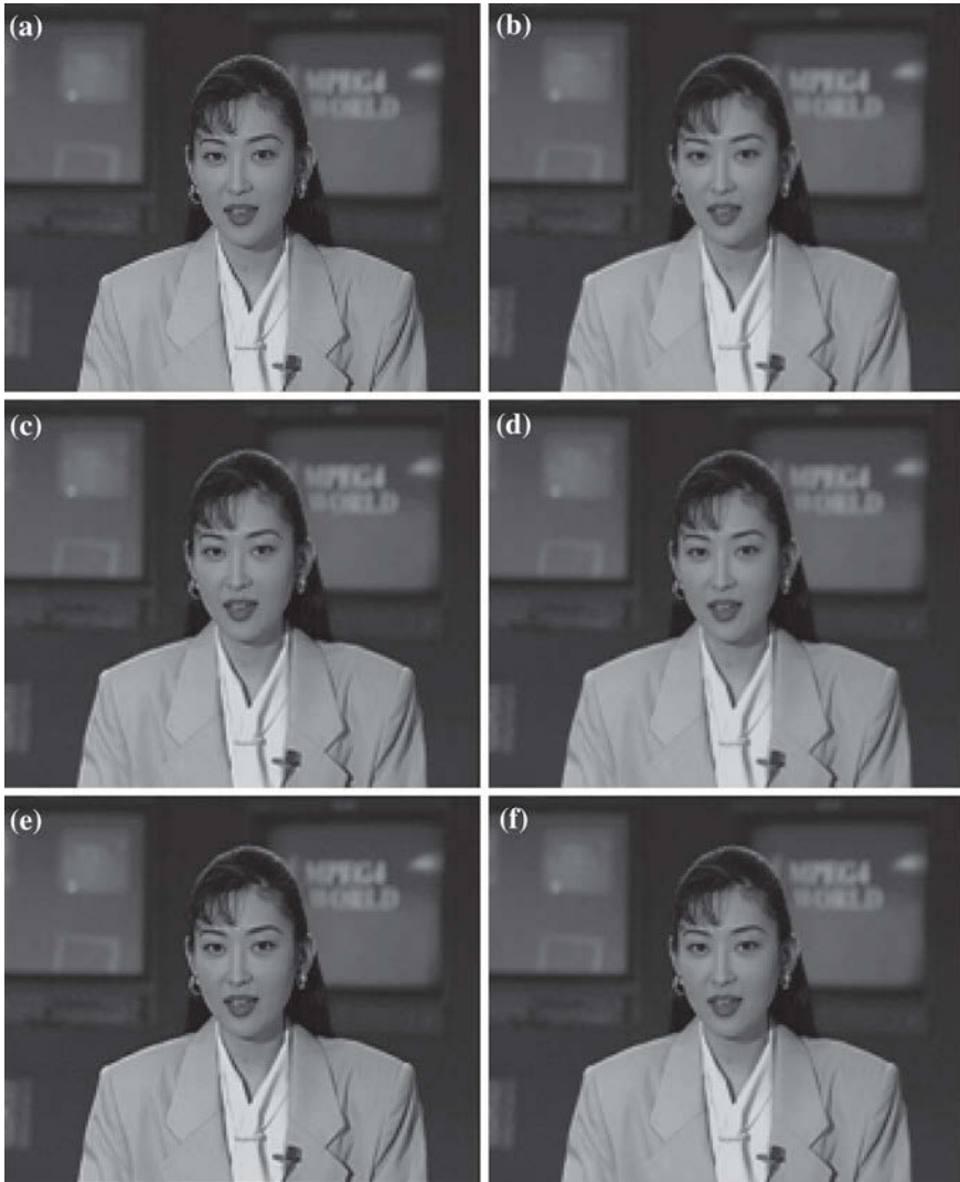
Fig. 10 Subjective performance of the 20th frame of the akiyo sequence at 4:1 compression ratio using different interpolation techniques: a Original, b Bicubic, c Lanczos-3, d DCT, e Crisp-rule based Lanczos-3 (Proposed-1), f Fuzzy-rule based Lanczos-3 (Proposed-2)
