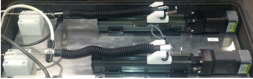
Fig. 3 Respiratory channels with pneumatic pressure sensors attached
