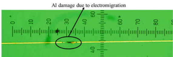
Fig. 13 Microscope image of the damage due to electromigration in the Aluminum track
