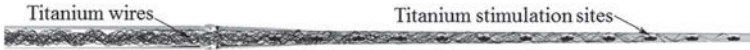
Fig. 3 An uncurled electrode array from MED-El coated with silicone, making the device flexible [5]
