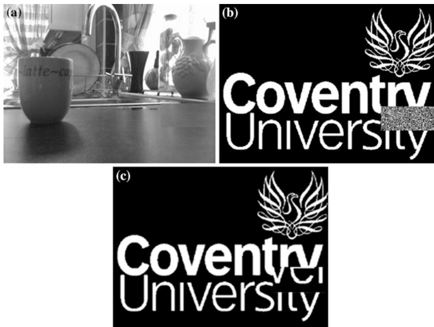
Fig. 18 Evidence of image tampering via the watermark; a Watermarked grayscale image, and b Watermarked LSB showing signs of tampering with an un-watermarked image, and c Watermarked LSB showing signs of tampering with another watermarked image
