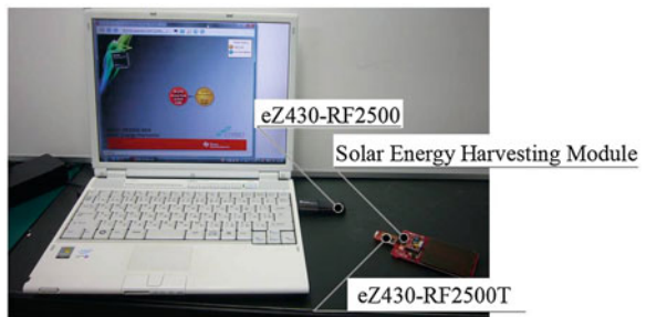
Fig. 3 Demonstration setup with wireless power transmission and sensor monitor
