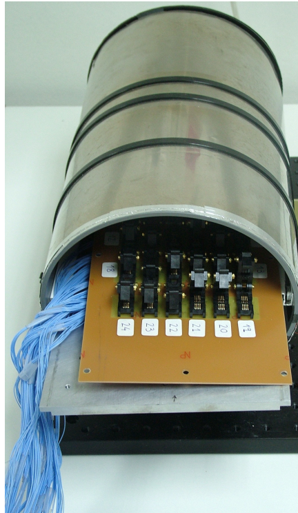
Fig. 15. PCB with sockets inside the one-layer mumetal shielding chamber
