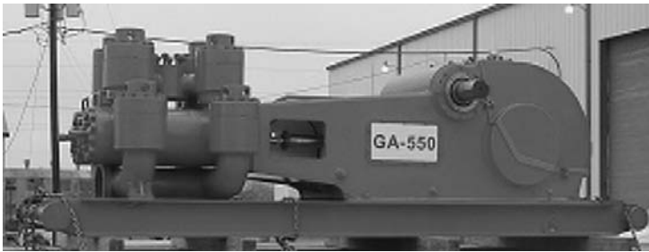
Figure 1.2 A duplex pump. (Courtesy of Great American.)
