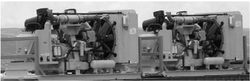
Figure 5.5 Air Drilling Specialties IR-XHP1170FSCAT compressor.
