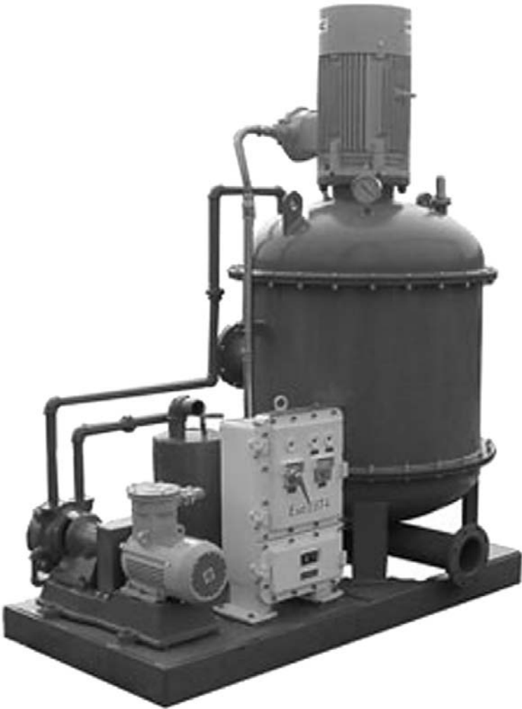
Figure 1.14 A vacuum degasser. (Courtesy of TSC.)
