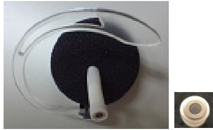
Fig. 3. Ear-worn temperature sensor (left) and its sensing part (right)
