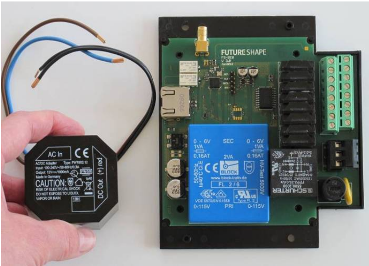
Fig. 10. The built-in power supply for the SensFloor underlay (left) and the SensFloor transceiver (right) for the controlling of Ambient Assisted Living applications. It features eight relays for 230 Volt devices, 2 potential-free relays, as well as a serial interface.
