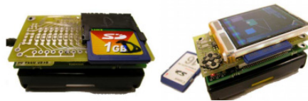
Fig. 7. The sensor nodes capable of in-network storage using an external SD/MMC storage device, which is implemented based on the MICAz mote [51]
