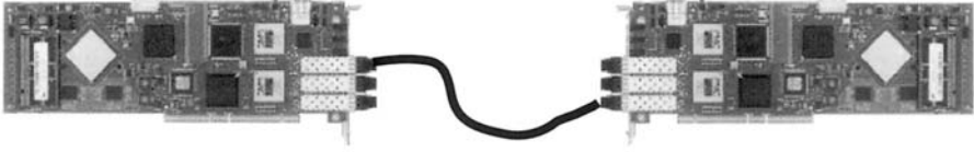
Fig. 4. Testbed 1: Measuring the maximum performance of PktGen.
