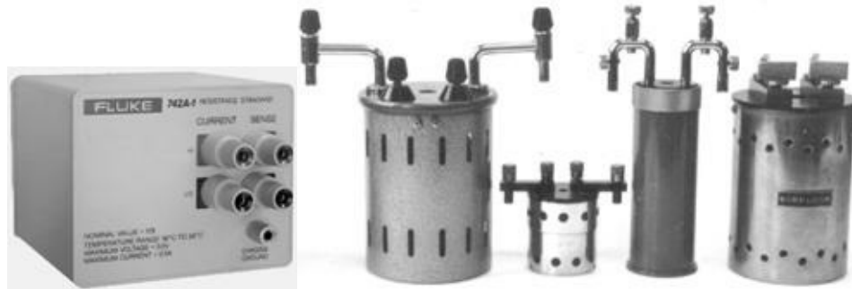
Figure 3.7 Resistance standards of different types in the Primary Electromagnetic Laboratory of Croatia (from left to right: Fluke, VEB, Guildline, Leeds&Northrup and Siemens&Halske)
