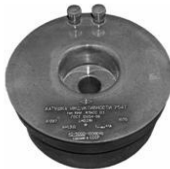
Figure 3.21 Inductance standard of 0.01 H
