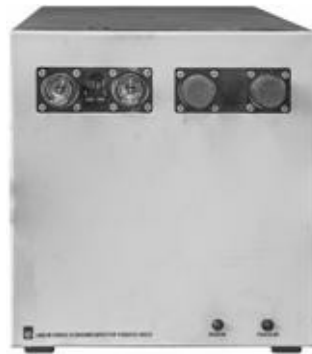
Figure 3.18 Usable standard capacitor 100 pF (Primary Electromagnetic Laboratory of Croatia)
