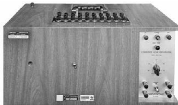
Figure 3.24 Weston cell standard at the Croatian Primary Electromagnetic Laboratory
