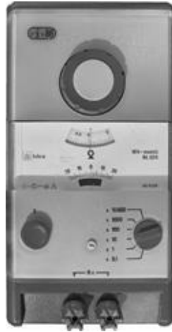
Figure 5.3 Commercial Wheatstone bridge
