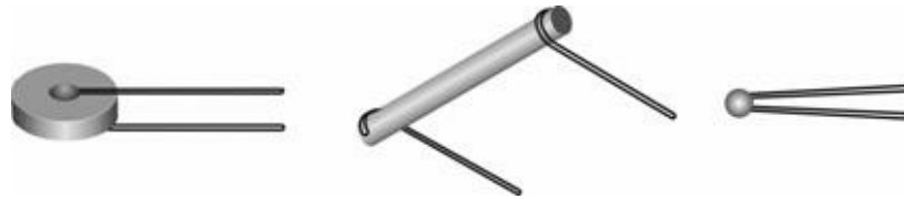
Figure 12.7 Types of thermistors
