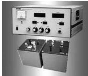
Figure 10.47 Commercial Schering bridge
