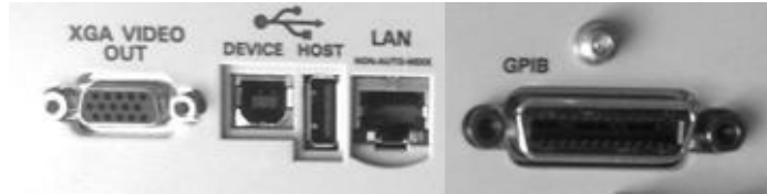
Figure 11.9 Modern oscilloscope with LXI (LAN), USB, GPIB, and video connectivity
