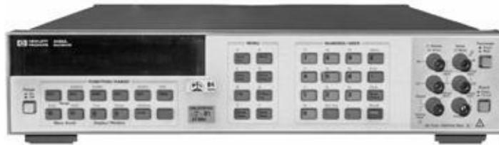
Figure 9.1 Precision voltmeter Agilent 3458A with 8 ½ digit resolution at the Faculty of electrical engineering and computing in Zagreb
