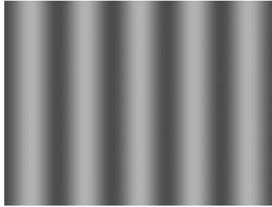
FIGURE 2.8 A simulated optical system's output (image), given the sinusoidal test object of Figure 2.6 as the input. Note that the spatial sinewave input is attenuated by the system's MTF. Peak contrast is also reduced.
