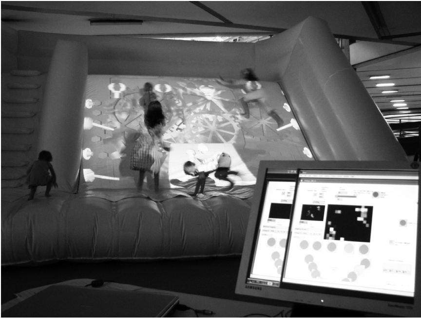
FIGURE 7.3 Robot Factory with a group of very young children using the ramp to climb. In the foreground the screen shows the computer vision control system that the 'host users' use to verify that the activity of the 'guest users' is adequately tracked and that the elements of the virtual environment are being correctly activated by them.
