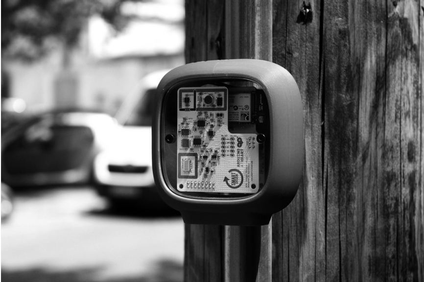
FIGURE 3.1 Smart Citizen Kit. Photograph courtesy of Smart Citizen.
