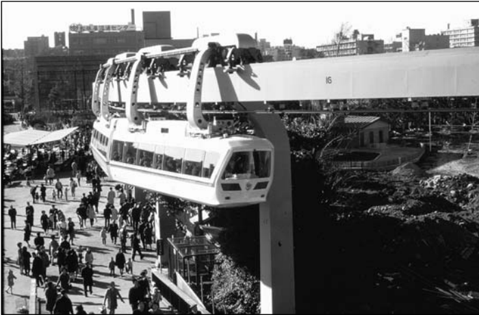
Suspended monorail linking a recreational area to rapid transit in Tokyo.
