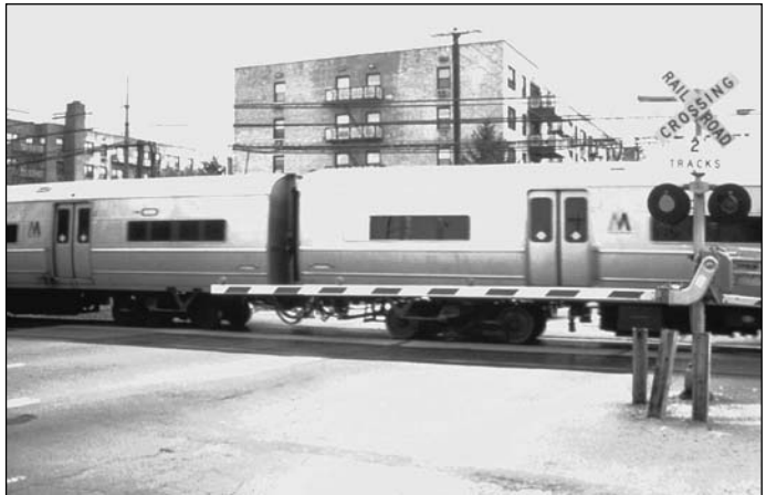
Protected grade crossing on Long Island.
