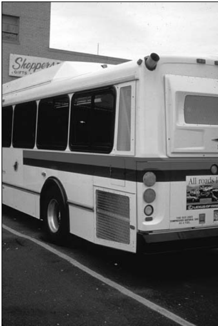
Bus powered by natural gas (tank on top).
