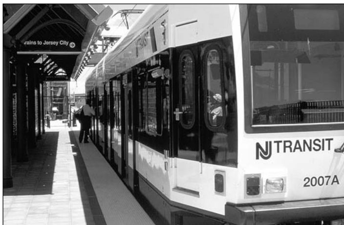
The low-floor Hudson-Bergen light rail vehicle and station in Jersey City, New Jersey.
