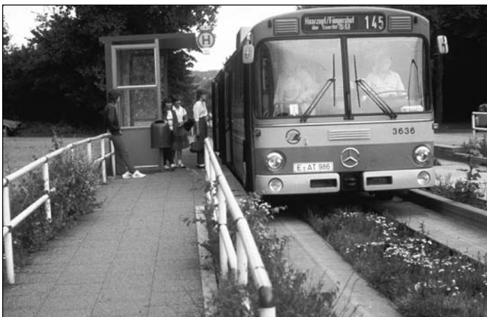
The O-Bahn (guided bus) track and stop in Essen, Germany.
