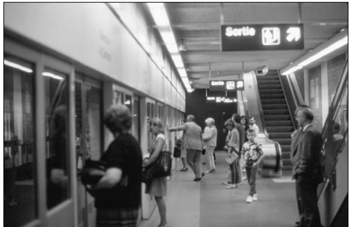
VAL system in Lille, France, employing platform edge barrier.
