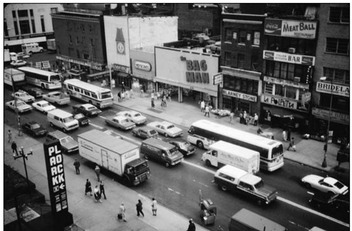
High-density traffic on 34th Street in New York City (level of service F).
