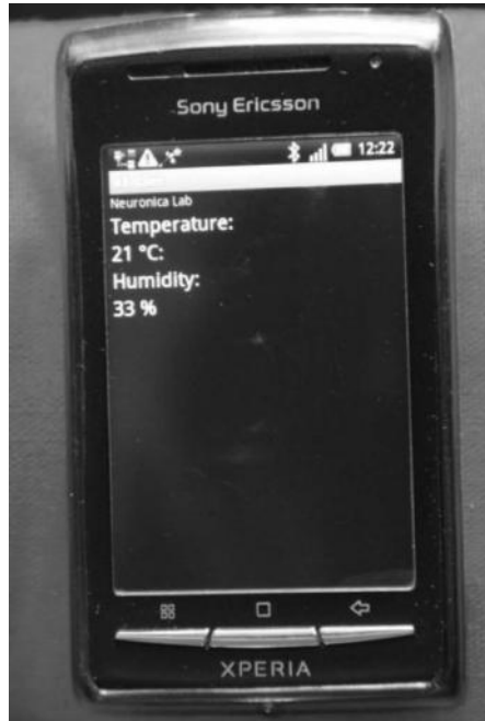
FIGURE 73.3 The “Display” part of the aBluSen previous version shows the temperature and humidity values obtained from the Bluetooth-based acquisition system.
