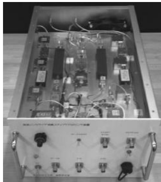
FIGURE 62.2 Stepped-FM UWB sensors: (a) Block diagram, (b) signal waveforms, and (c) external photo of setup.
