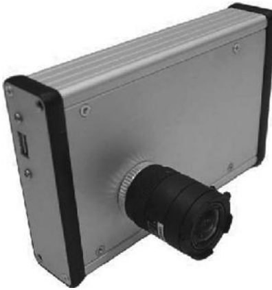
FIGURE 4.23 SCAMP-3 programmable vision chip.
