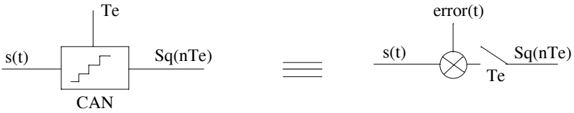
Figure 6.1. Modeling an analog-to-digital converter
