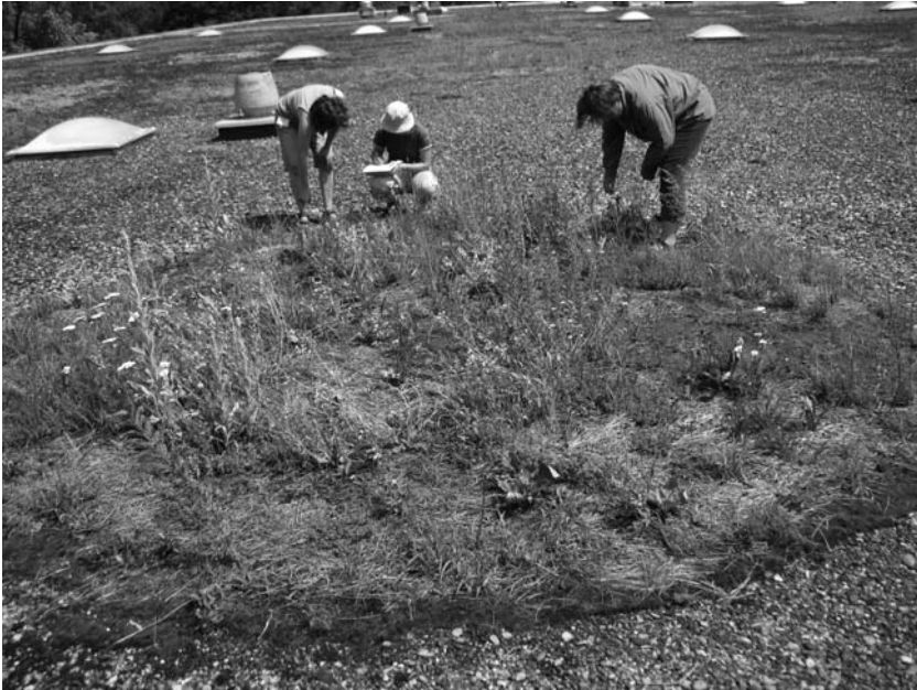
Figure 18.5 In July 2008, students from our department classified the plants and their cover percentage on the Rotkreuz roof during their environment analytics project week (from Chr. Groefflin (2008) with permission).
