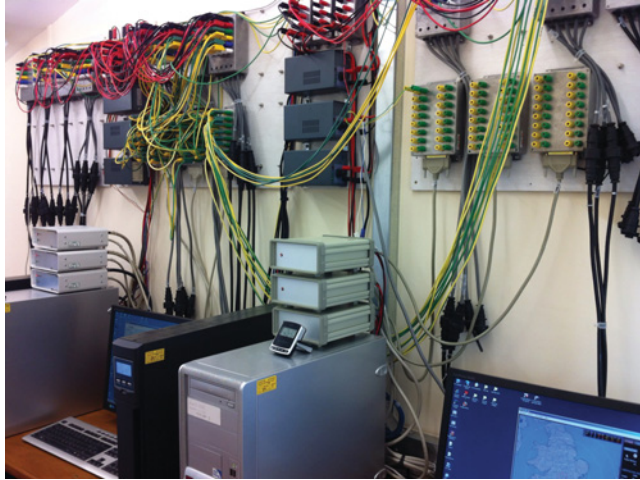
Figure 4.7 Multiple-channel data acquisition system used at Reading University Atmospheric Observatory, based on data acquisition cards connected to a standard desktop PC, which is also networked for web access to the data. The patchboard of wires allows the channels to be configured to the instruments connected.
