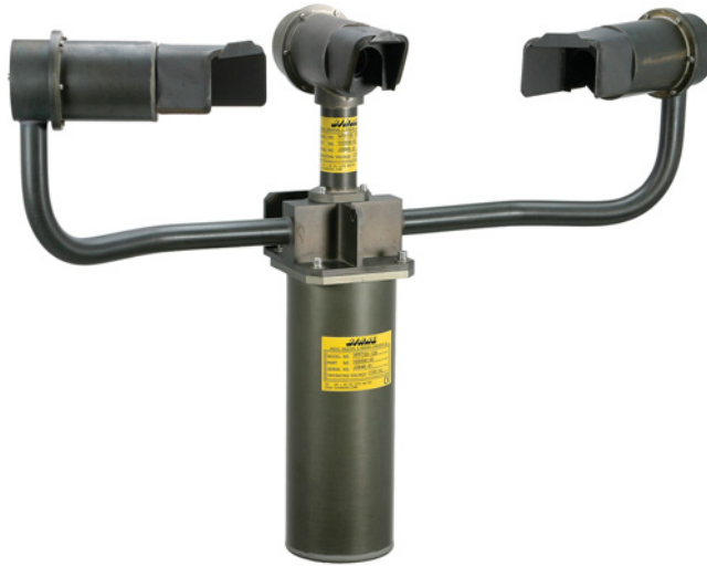
Figure 10.2 A combined visual range and present weather sensor. The left to right infrared beam is used to determine the visual range, and the third sensor used to discriminate between droplets, ice and snow.
