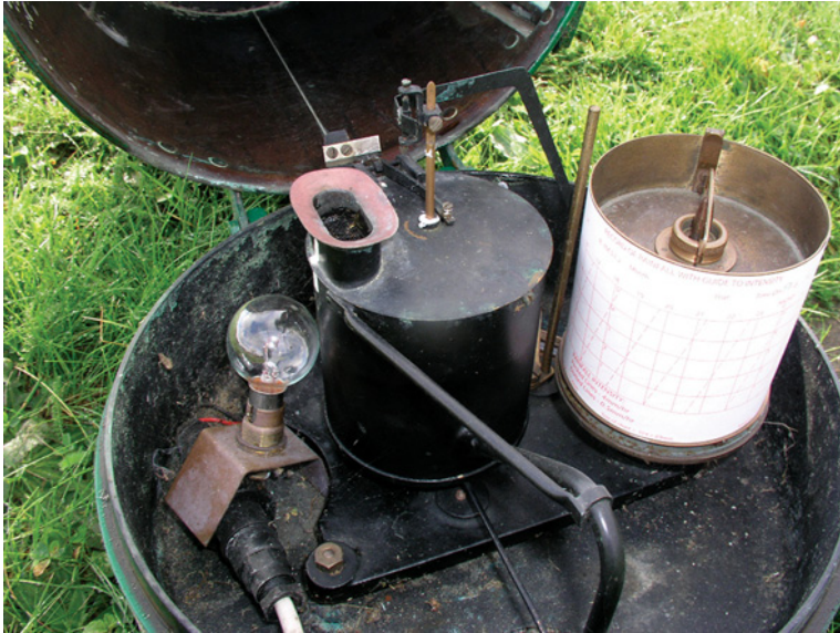
Figure 10.4 Tilting siphon rain gauge. The rain falls into the float chamber in the centre, and the position of the float determines the position of the pen on a recording chart, normally changed daily. When full, the chamber is emptied by a siphon action.
