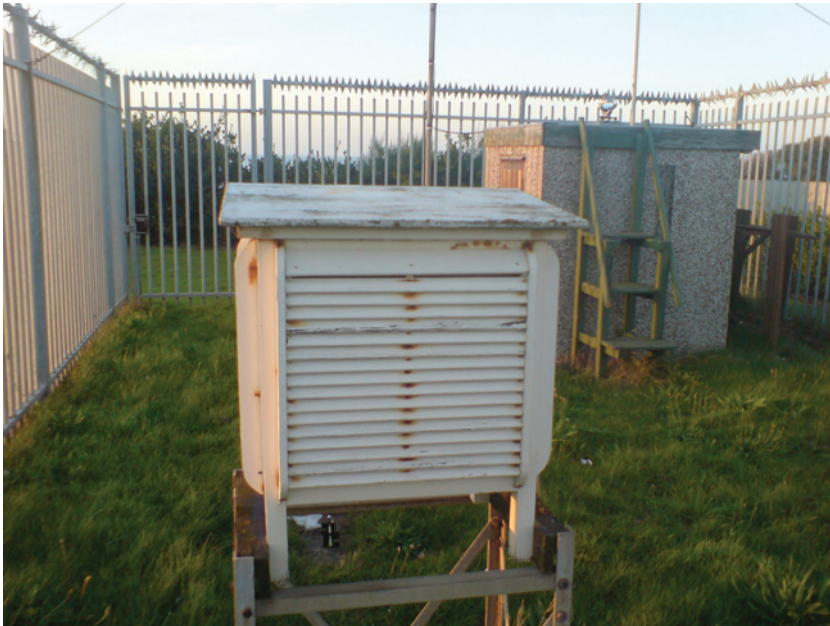
Figure 5.22 Thermometer screen used for climatological observations at a seaside resort.
