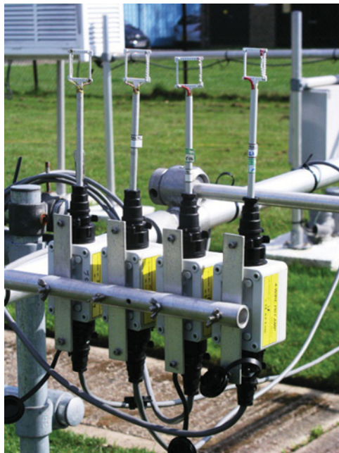
Figure 5.9 Array of fine wire resistance thermometers arranged for an air temperature comparison. The signal conditioning electronics is mounted in the box at the base of the thermometer. This minimises the effect of connection resistances, but still requires good thermal stability of the electronics.
