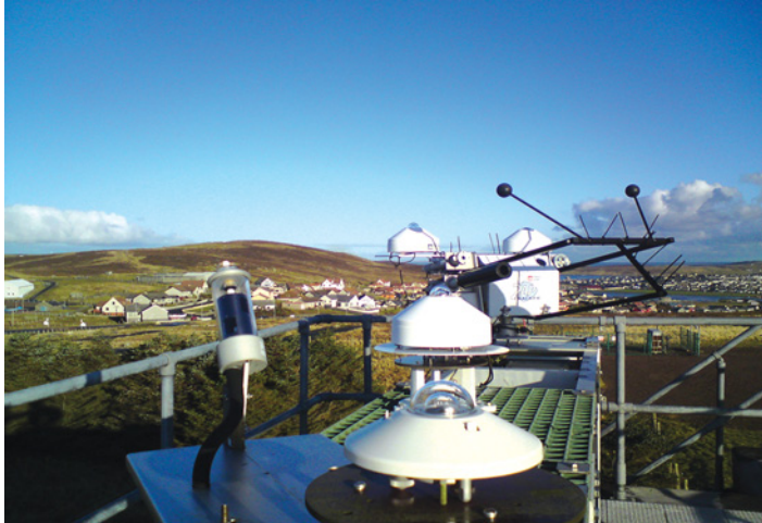
Figure 9.12 Solar radiation sensors in use at Lerwick Observatory, Shetland. In the foreground and background, four pyranometers can be seen. The two pyranometers in the background are mounted on a solar tracker, shaded by black spheres to allow diffuse radiation measurements. Beneath the two diffuse radiation pyranometers on the solar tracker is a cylinder pointing towards the sun, which houses the pyrheliometer. (The instrument in the foreground on the left-hand side is a sunshine recorder.)
