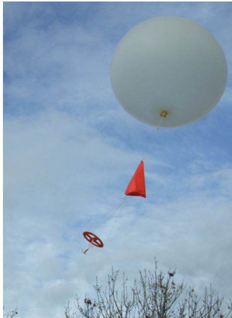
Figure 11.1 Sounding balloon just after launch, carrying a radiosonde instrument package (out of view). Beneath the balloon is a parachute, used to control the descent after the balloon bursts.
