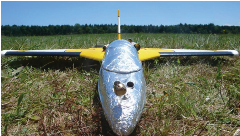
Figure 11.17 View of a small UAV carrying sensors for atmospheric measurements. An electrode to measure charge is mounted on the nose of the aircraft, and temperature sensors are carried within tubes visible alongside the fuselage above the wings. On the wings (not visible), are photodiode solar radiation sensors. (Approximate platform specifications: fuselage diameter 10 cm; wingspan 1 m; ceiling 4000 m and flight endurance 20 min.)
