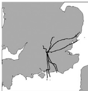
Figure 11.13 Examples of trajectories of radiosondes launched from Reading, up until the telemetry was lost or became intermittent. (The radiosonde position was determined using GPS information and the height calculated from the radiosonde pressure measurement.)
