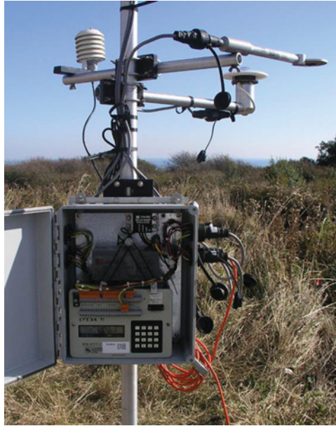
Figure 4.1 Photograph of an environmental data logger, deployed within a weatherproof enclosure. A range of environmental sensors measuring wind speed, temperature and radiation has been connected.
