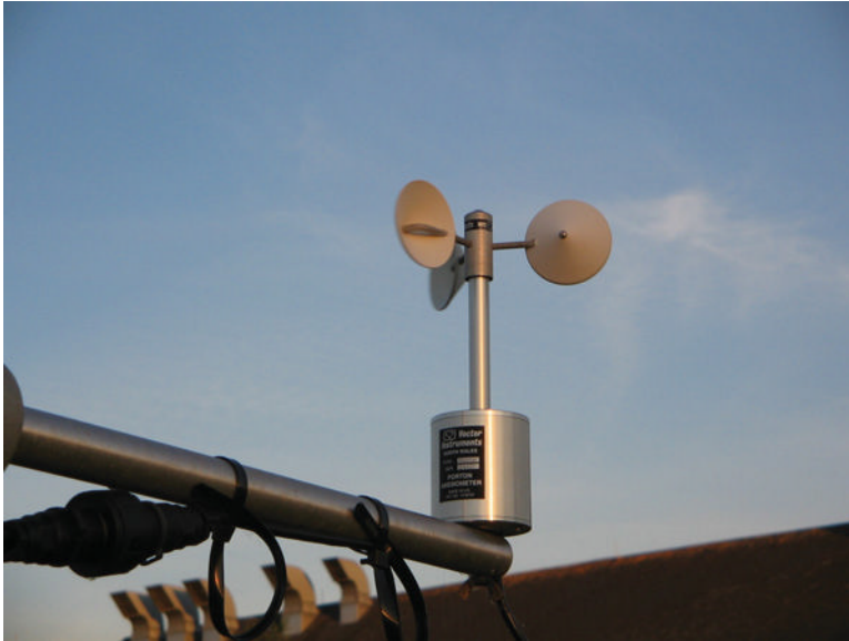
Figure 8.1 A three-cup anemometer used to measure the horizontal wind speed.
