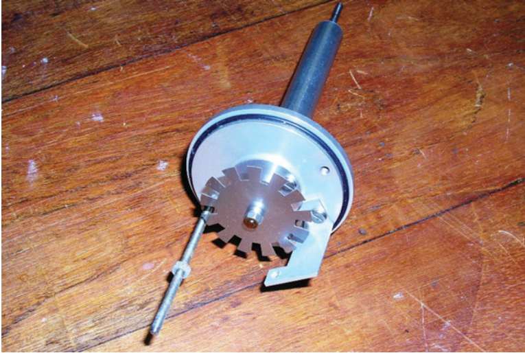
Figure 8.2 View of the optical shutter arrangement used in the lightweight cup anemometer of Figure 8.1. As the shaft rotates, a light beam between an optical source and electronic detector is regularly interrupted by the teeth on the shutter, generating a series of digital pulses at a rate which is proportional to the rotation speed.
