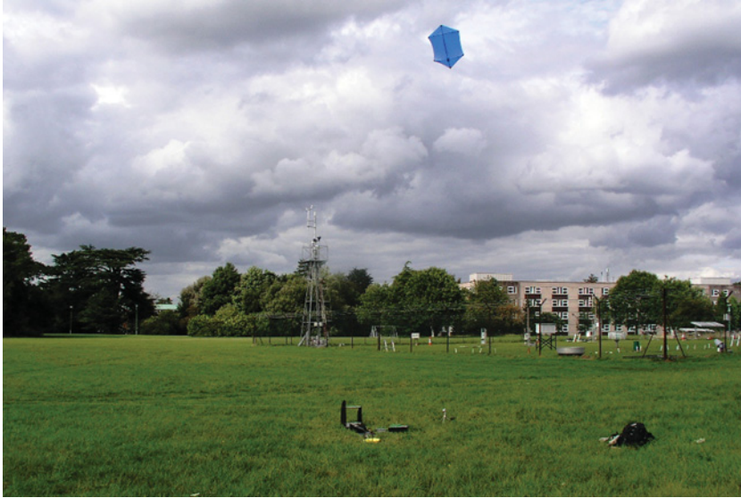
Figure 8.14 A Rokkaku kite (flat area 2.3 \text{ m}^2 ) with a tension-measuring sensor at the base of the tether, flown close to a sonic anemometer operating at 10 m.
