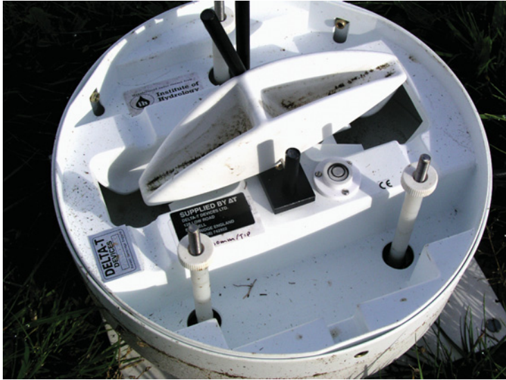
Figure 10.5 Tipping bucket mechanism within a rain gauge. The rain is collected in a funnel and falls onto the uppermost bucket of the two mounted on the sea-saw mechanism. When full, the mechanism tips, emptying the bucket and allowing the other bucket to fill. Each trip action operates a switch, generating a pulse.
