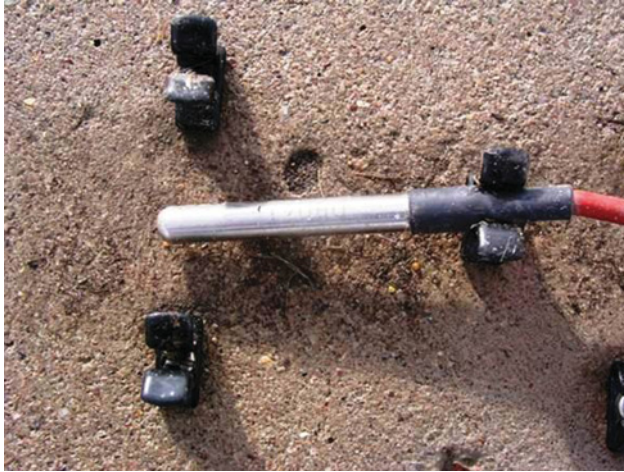
Figure 5.7 Platinum resistance thermometer (resistance element enclosed within a stainless steel sheath, 8 mm diameter), used to measure the temperature of a concrete surface. (In use, a half-cylinder radiation shield is fitted into the clips.)
