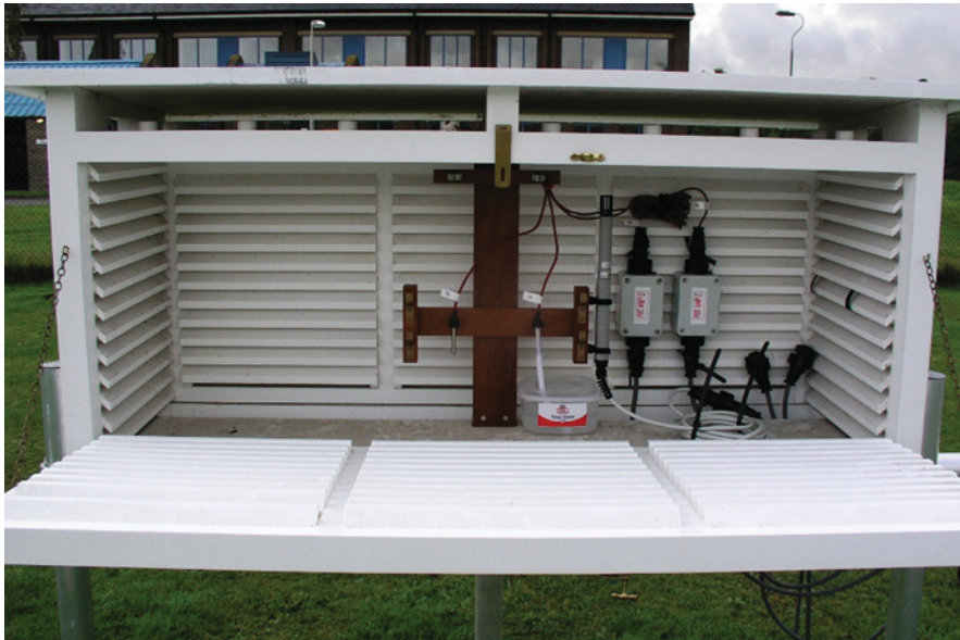
Figure 6.15 View of a psychrometer arrangement within a large thermometer screen. The two temperature measurements in the centre are obtained using platinum resistance sensors, the right one of which has a cotton wick attached to form a wet bulb thermometer.
