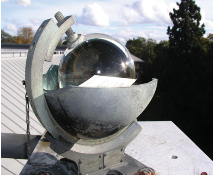
Figure 9.32 A Campbell–Stokes sunshine recorder.
