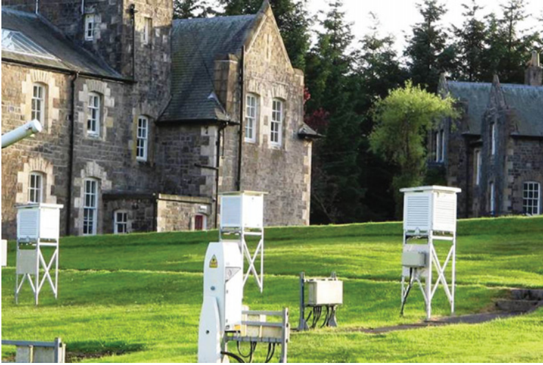
Figure 5.16 Stevenson screens in use at Eskdalemuir Observatory, Dumfriesshire.
