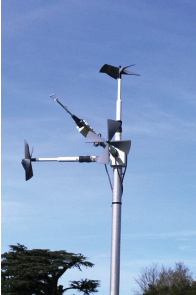
Figure 8.3 An array of three orthogonal propeller anemometers providing a rapid response to wind fluctuations, from which the wind direction can also be found. (A fast response thermometer is also mounted in the middle of the anemometer array.)
