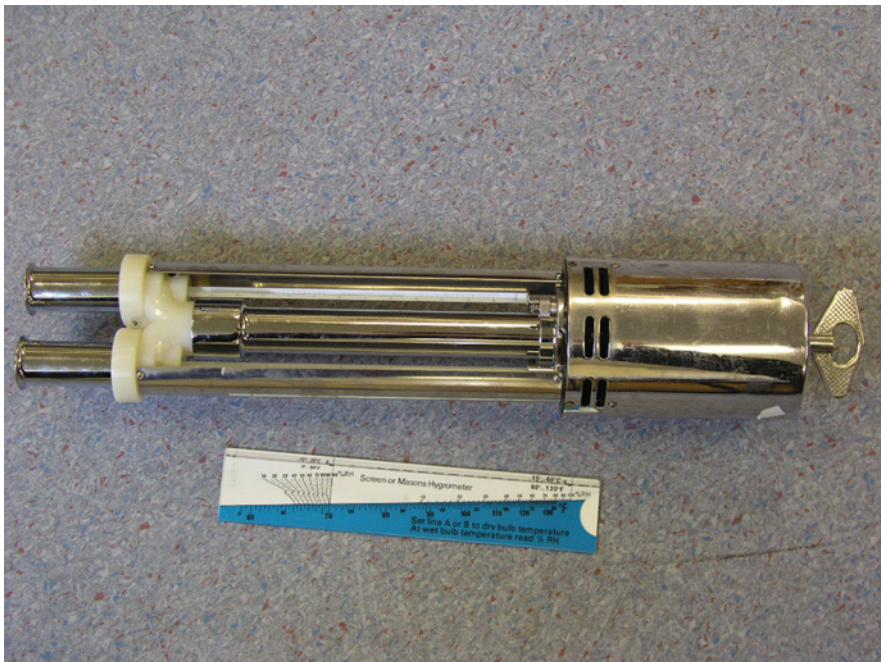
Figure 6.14 An Assmann psychrometer. This uses polished metal shields to protect the thermometers from radiation, and applies forced ventilation by a clockwork motor.
