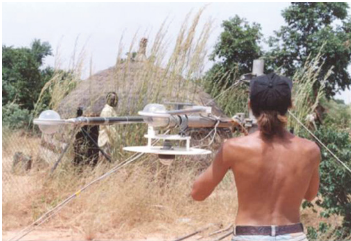
Figure 9.28 Use of pyrrometers (and a downward facing pyranometer) at a remote site in the Sahel. The pyrrometers use upward and downward polythene domes for protection, inflated by dry air from a pump.
