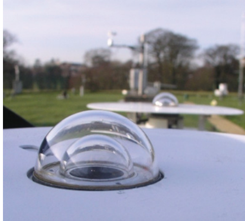
Figure 9.8 Pyranometers installed at Reading Observatory, showing the protective glass domes and white body shielding.
