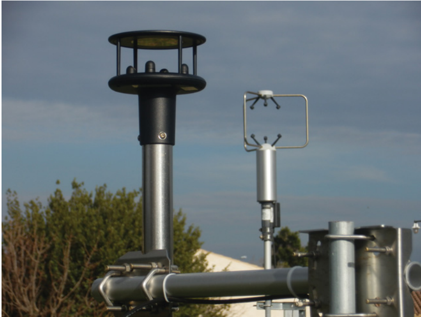
Figure 8.7 Ultrasonic anemometers mounted on masts. In the foreground is a two-dimensional device, and in the background a three-dimensional device. For the three-dimensional anemometer, the three pairs of transmitting and receiving transducers are towards the centre, with an outer support frame arranged to minimise disturbance to the flow.
