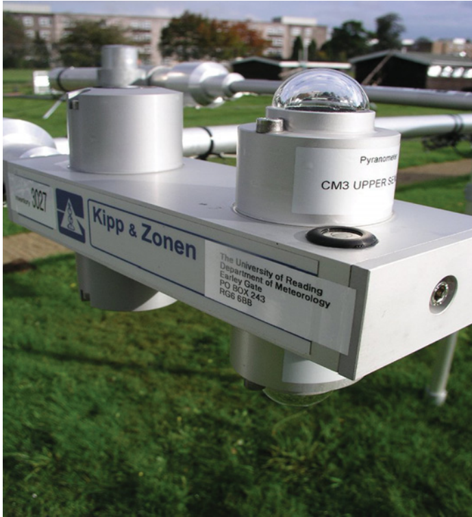
Figure 9.30 A four-component net radiometer, measuring the upwelling and downwelling shortwave radiation (domed sensors), and the upwelling and downwelling longwave radiation.
