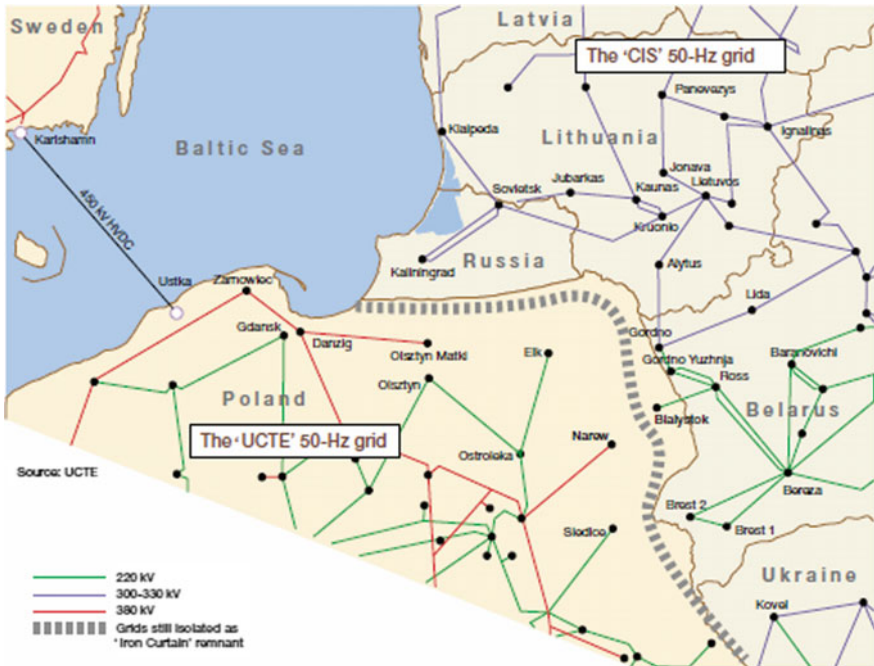
Fig. 6.7 Baltic electric power generating ring
