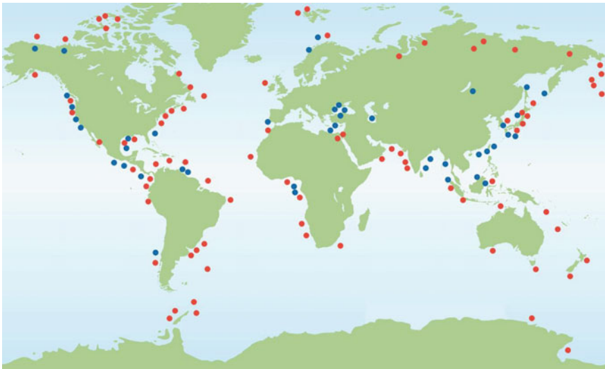
Fig. 3.12 Location of deposits of GH (Blue dots the places where the presence of GH exploration drilling confirmed, red dots confirmed indirectly by geophysical exploration)
