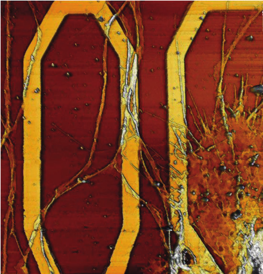
Fig. 8.17 A neuron cultured on an electronic chip. The chip is designed to pick up an action potential from the cell. The image demonstrates the proper tracing of the cell surface. In a future application, an appropriately designed stylus could be used as an additional electrode to excite or record an action potential at any location on the cell body or a neuronal cell process
