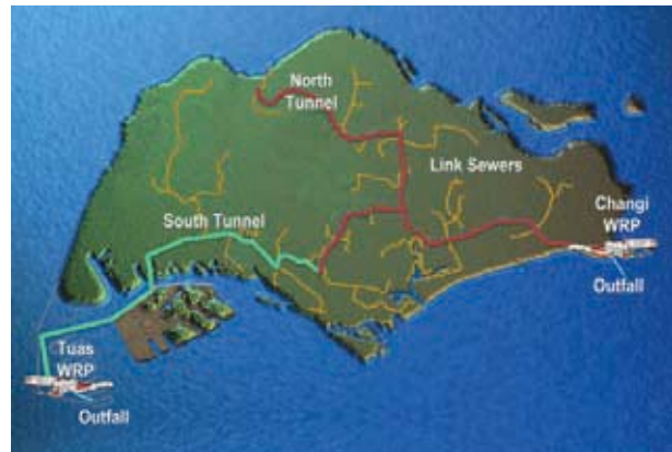
Figure 8 The Deep Tunnel Sewerage System
