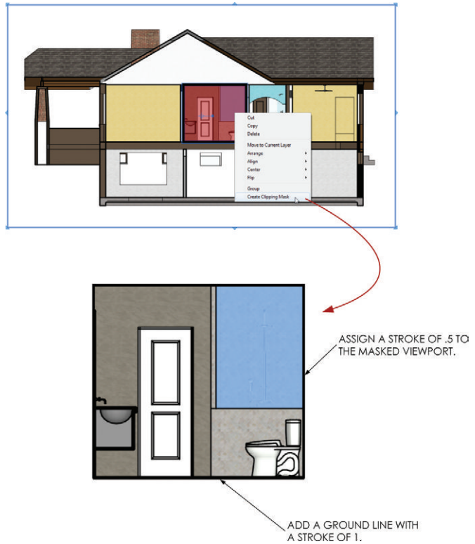
Figure 20.27 The interior elevation
