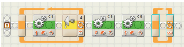
Fig. 4. Incorrect use of the second loop: putting the loop after the initial program
