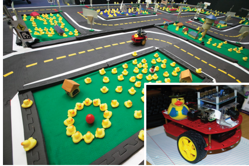
Fig. 1. Duckiebots are minimal autonomy platforms designed to operate in Duckietowns of arbitrary topology.
