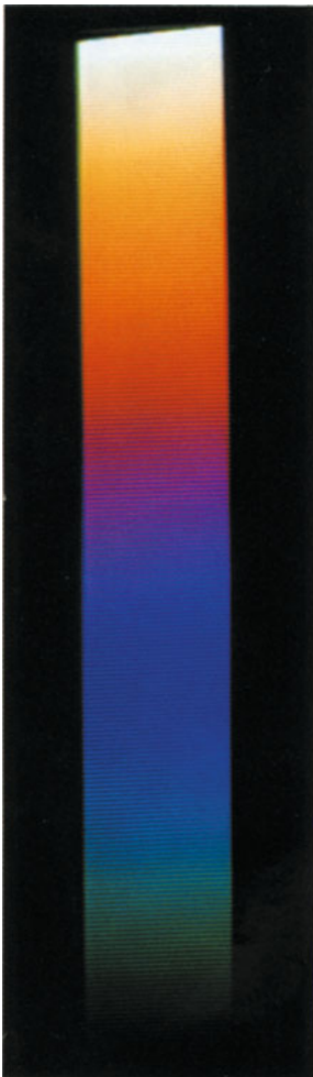
Fig. 5.1. The colour scale used to display all images in this book. Each pixel is displayed with a colour corresponding to the number of counts it contains. The top and bottom colours of the scale are assigned to the maximum number within the set of tomograms and to zero respectively.
