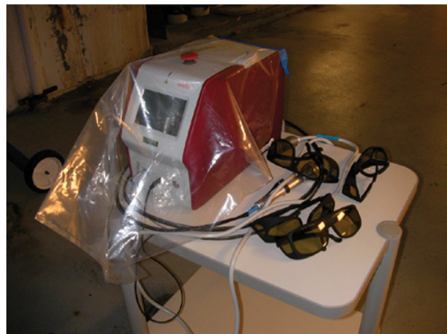
Figure 29.2 Protective plastic cover to prevent water splashing on the laser.
