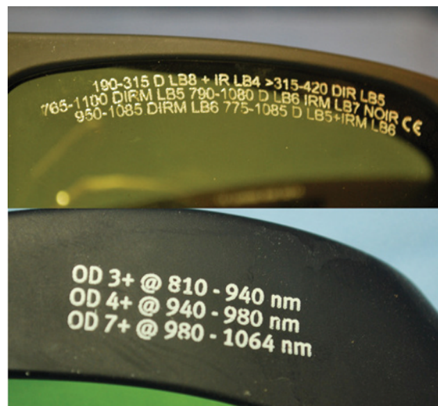
Figure 4.2 Specification of wavelength and OD on the lens (top) and frame (bottom).
