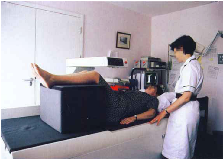
Figure 4.6 A currently used DXA instrument. The fully-dressed subject lies above the dual X-ray source and below the mobile detector.
