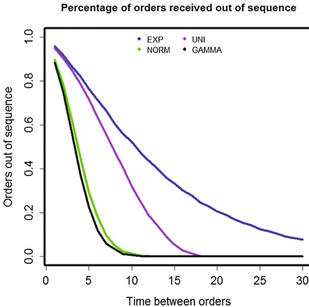
Fig. 2. Likelihood of order crossover occurring for the four distributions as a function of the time between orders.
