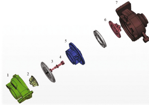
Fig. 3. Turbocharger expanded view [12].
