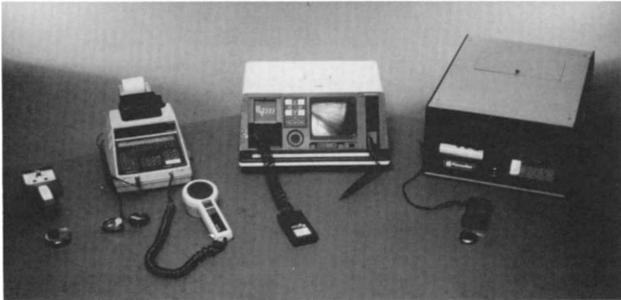
Figure 3.3 Pacemakers with their programmers. As pacemakers became smaller and more sophisticated their programmers became large and complex (left to right)
