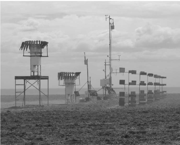
Figure 3: Instrumentation to measure soil and PM10 loss from a field during summer fallow within the Columbia Plateau.
