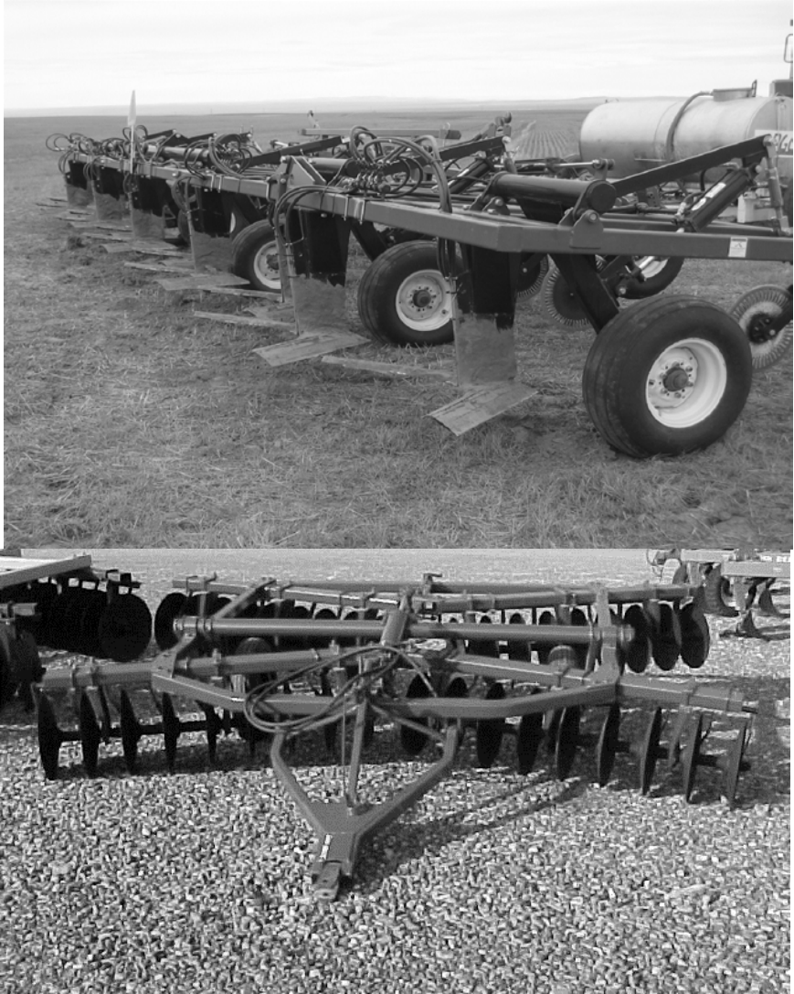
Figure 4: The top image is an undercutter tillage implement with 0.8-m wide V-blades and the bottom image is a conventional disk implement.
