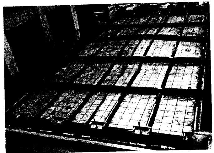
(c) OVERALL GRILLAGE BUCKLING (MODE 4)
