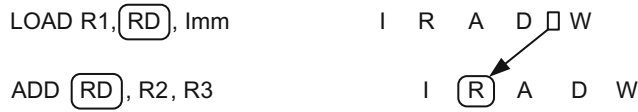
Fig. 6.70 A forwarding path to remove the data hazard caused by the LOAD instruction followed by a register-type instruction
