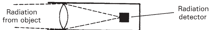
Figure 13.6 Structure of a radiation pyrometer. From Morris (1997) Measurement and Calibration Requirements , © John Wiley & Sons, Ltd. Reproduced with permission.
