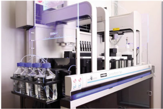
Fig. 1 The Patchliner and SyncroPatch 384PE instruments. (a) The Patchliner pipetting robot with borosilicate glass chip located inside the measure head. Computer and amplifiers required for running the system are not shown (reproduced with permission from [12]). (b) The SyncroPatch 384PE recording module with borosilicate glass chip located outside of the measure head. (c) The SyncroPatch 384PE located inside the Biomek FX ® (Beckman Coulter) during a recording. The glass bottles containing internal solution and the pipettor with 384 pipettes can be seen. (d) The 384 pipetting head of the Biomek FX ® shown positioned inside the chip while dispensing solution to the chip ( b–d , reproduced with permission from [20])
