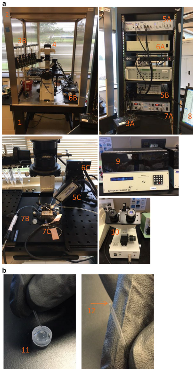
Fig. 4 (a) Manual patch-clamp setup for APD measurements with a glass culture dish on the heater adapter under the microscope. 1, Air table; 2, Faraday cage; 3A, solution perfusion controller; 3B, syringe reservoirs for vehicle and test compound storage and perfusion; 4, inverted microscope; 5A, Axon MultiClamp amplifier; 5B, digitizer; 5C, headstage with pipette holder; 6A–C, micromanipulator; 7A, dual channel heater controller; 7B, inline solution heater; 7C, cable assemblies with connector for heater adapter for dish; 8, computer; 9, pipette puller; and 10, microforge. (b) Image of glass pipette being backfilled with intracellular solution using the cap of screw cap tube. 11, Backend of glass tube (non-pulled end); 12, arrow points to a small bead of intracellular solution at the pipette tip
