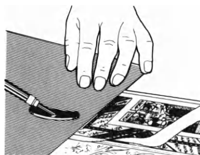
Figure 2.70. The leaf is laid onto a silicon paper protected board. The repair is attached loosely using a heated spatula through a silicon paper barrier.
