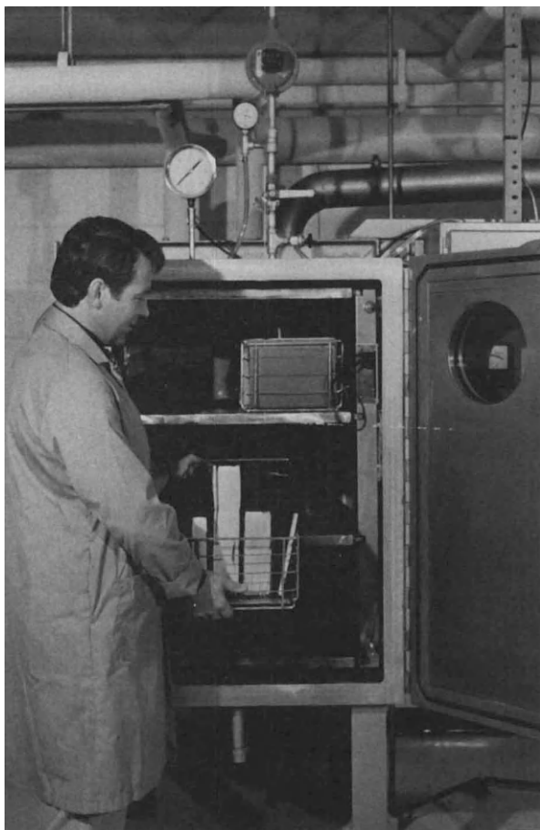
Figure 2.94 shows R. Couture, system operator, removing a basket of dried books from the Stokes vacuum drier. Twelve baskets of books are expected to be transferred into the vacuum dryer each evening and brought to a temperature of 140°F (66°C) and a high vacuum overnight. The paper in these vacuum-dried books is thoroughly dry. Contrary to conventional opinion, this bone-
