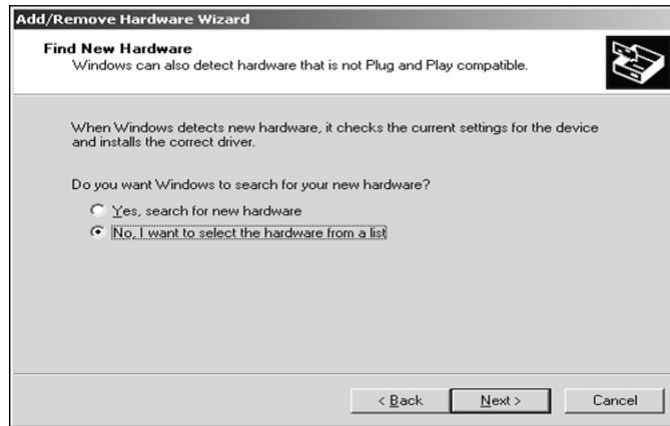
Figure 6.7 Choose the No Option to Select the Device from a Hardware List
