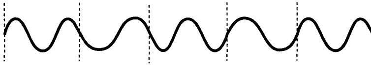
Figure 4-9 - FFSK carrier waveform for space = 7,500 Hz, mark = 12,500 Hz, data rate is 10,000 baud. The figure represents the binary sequence 10101
