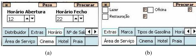
Fig. 5. Query device based on (a) numericUpDown control for range selection values (b) checkboxes for multiple choice queries
