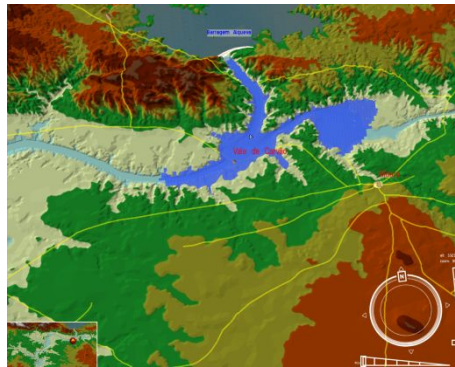
Fig. 2. Simulation of the flooding wave in the Guadiana River created by the failure of the Alqueva Dam
