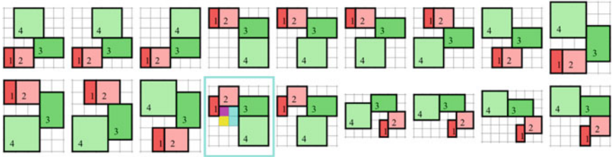
Fig. 1.16 18 potential solutions. Only one (indicated by a frame) is proper according to the criteria defined above. Magenta and cyan indicate the sub-corridors for the “red” and “green” apartments, respectively. Yellow indicates the main corridor which connects both sub-corridors. The total number of grid-cells occupied by the communication is four
