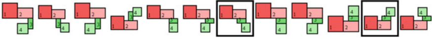
Fig. 1.13 Improved layouts as a result of additional geometrical constraints. Room configurations framed in black are in fact classified as “proper” according to so called “corridor criterion”
