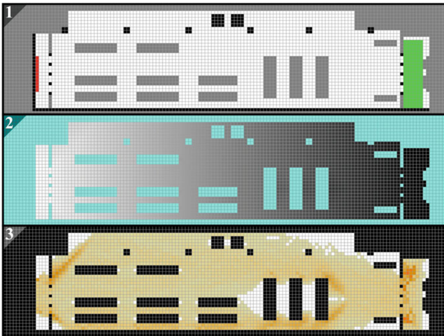
Fig. 5.2 1 The rescaled floor-plan ready for CS. A single pixel is equivalent to the 0.4 \times 0.4 m area corresponding to the size of an agent. The fixed and modifiable elements are shown in black and gray , respectively. Red indicates the exit cells. Green indicates the holding area where the initial positions of agents are randomly distributed. 2 A visualization of the combined DF for all exit cells. The closer is an exit, the brighter are the cells. Background is shown in cyan . 3 A visualization of the HM recorded at the preliminary simulation. Higher color saturation of cells correspond to more frequent visits of the agents. White indicates the unvisited areas
