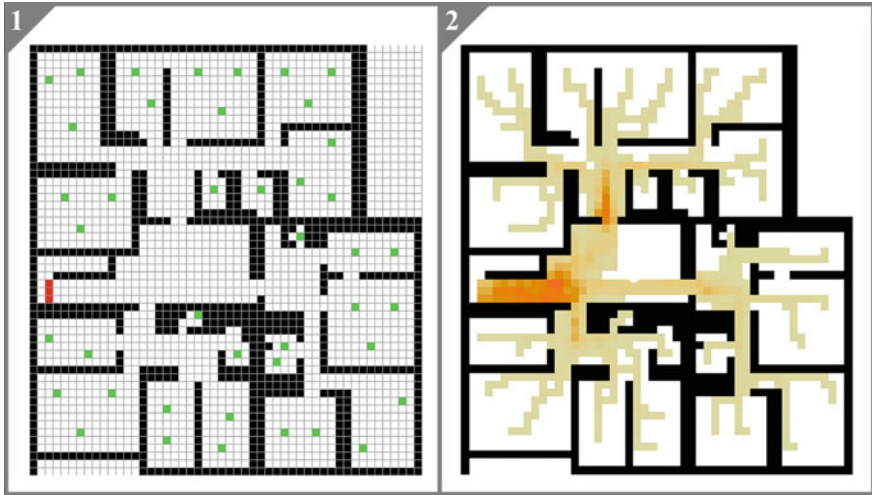
Fig. 3.20 1 The final CS environment with “manually” adjusted floor-plan. The initial positions of agents and exit cells have been also placed “manually” and are shown in: green and red , respectively. 2 Although HM indicates certain congestion at the exit, this floor-plan seems acceptable regarding safe evacuation
