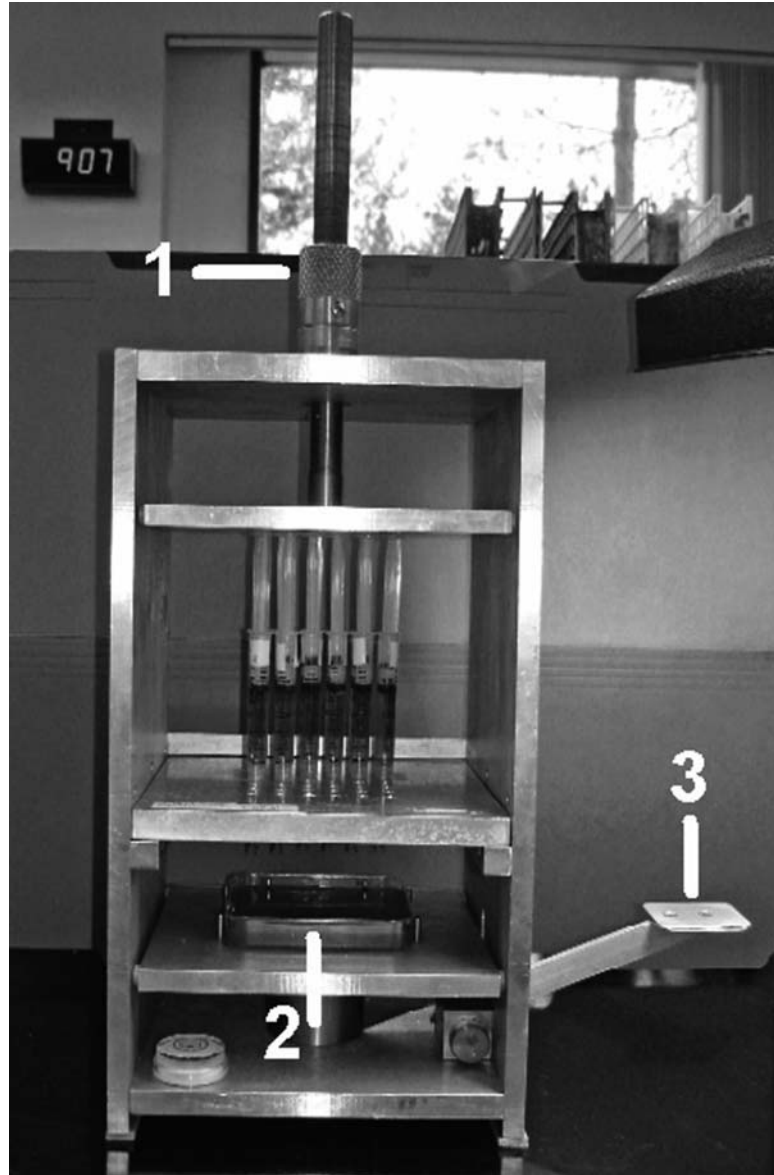
Fig. 17.1. Dispenser with phage-loaded syringes in place. Turning the knurled knob at the top (arrow 1) depresses the syringe plunger allowing small drops (see Fig. 17.2) to fall onto the plate (arrow 2). This is raised just below the cannulas by depressing the lever arm (arrow 3).
