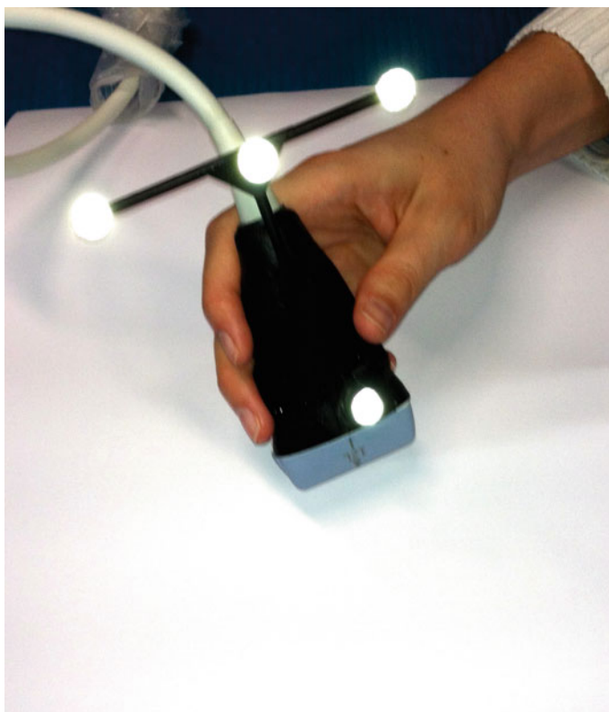
Fig. 1 Ultrasound transducer with a customized cluster composed by four noncollinear reflective markers fixed to the long axis of the transducer
