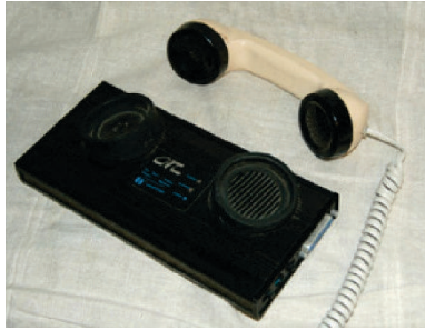
Figure 9.1 A Novation CAT acoustically coupled modem [4]. Source: Lorax on en.wikipedia (public domain): https://commons.wikimedia.org/wiki/File%3AAcoustic_coupler_20041015_175456_1.jpg
