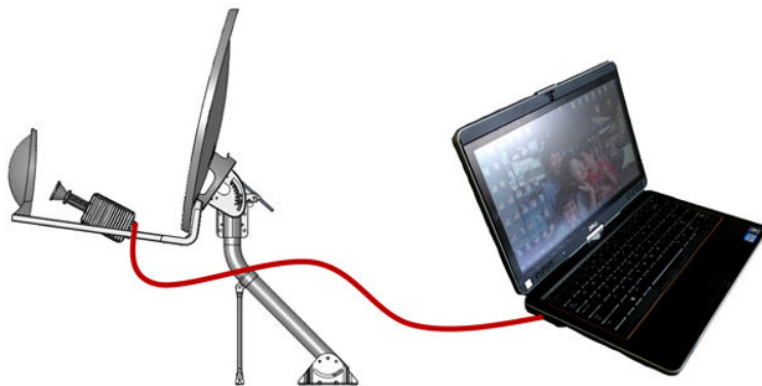
Figure 11.8 A typical VSAT terminal antenna connection. Source: Axlsite (own work) CC BY-SA 3.0 ( https://commons.wikimedia.org/wiki/File%3ATooway_satellite_antenna_drawing.png )
