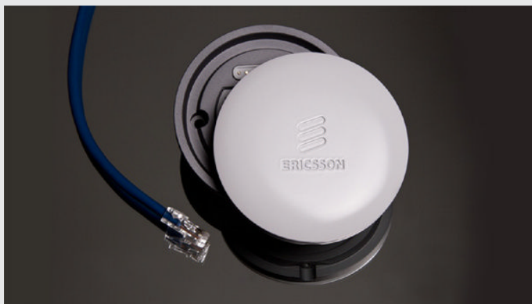
Figure 13.10 Radio Dot by Ericsson. Reproduced by permission of Ericsson AB [12]
