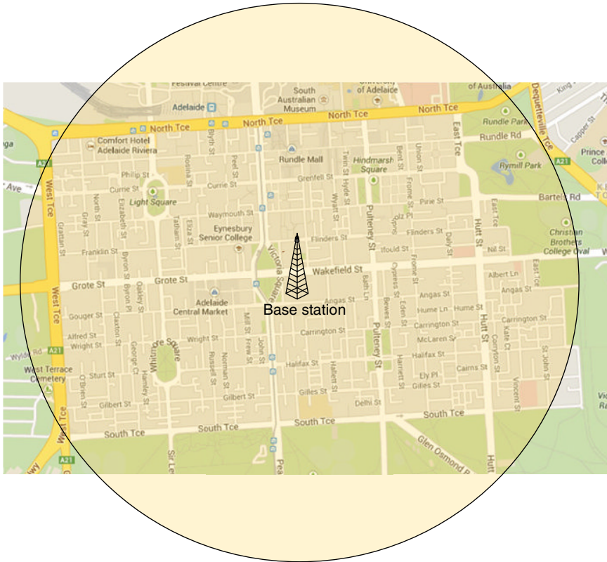
Figure 13.6 A possible initial coverage of Adelaide CBD using macrocells
