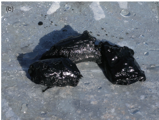
Figure 11.13 Monosulfidic black ooze in a benthic core (a) from a canal estate on the Peel-Harvey Estuary, WA, is black and gel-like (b). (Source: Leigh Sullivan.)
