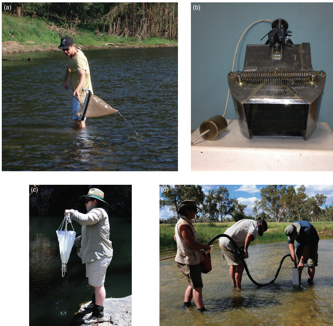
Figure 4.3 Different sampling equipment used to collect organisms from different habitats: (a) sweep-net sampling with a pond net (here, held above the water to show the collecting bag on the frame); (b) a benthic grab sampler, spring-loaded in the 'open' position and triggered shut when the heavy weight ('messenger' to the left) is released to slide down the cord and hit the top of the sampling box; (c) a plankton net, with a sample-jar screwed to the apex, about to be cast out into the water and towed back to shore; (d) a stove-pipe sampler (the middle person is using a bilge pump to evacuate the contents of the sampling box (right) into a collecting net (left)). (Source: (a) and (b) Darren Ryder, (c) and (d) Jenny Davis.)
