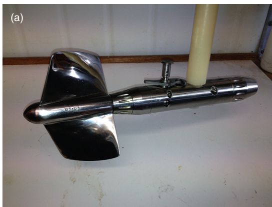
Figure 5.6 Current velocity can be measured using various meters: (a) a propeller design that counts revolutions of a spinning blade, (b) an electromagnetic meter that measures changes to the electromagnetic field around its bulb to estimate velocity. (Source: Darren Ryder.)
