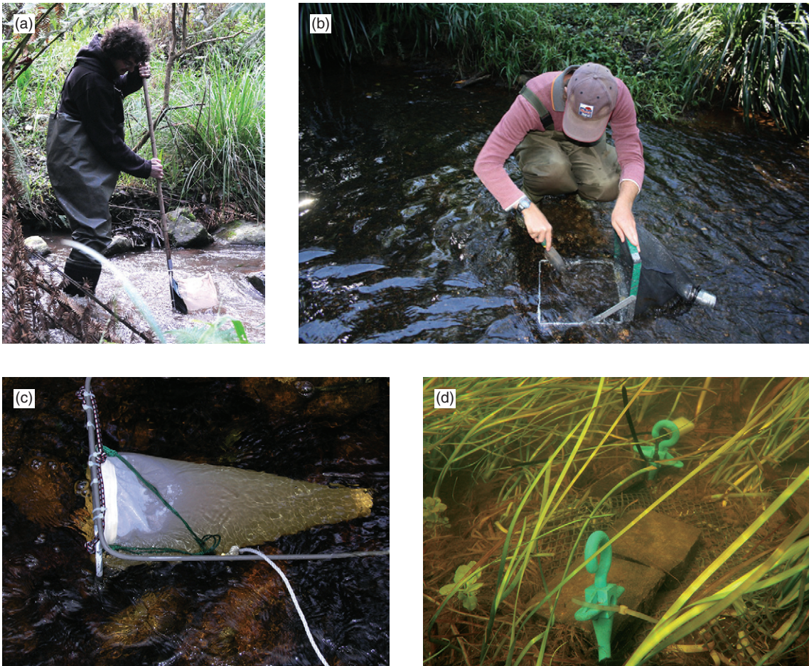
Figure 7.3 Habitats in flowing waters can be sampled using a pond-net (a), Surber sampler (b), drift net (c) or from artificial substrates (d). (Source: (a) Jenny Davis, (b) Judy Davies, (c) Belinda Robson, (d) Edwin Chester.)
