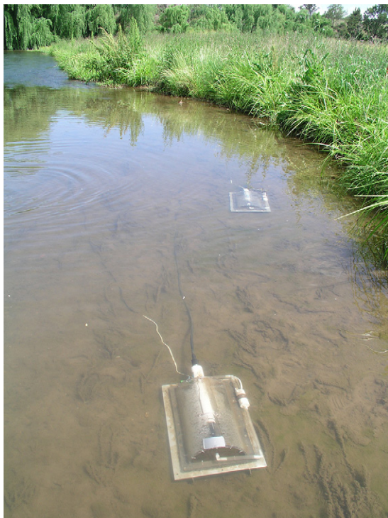
Figure 11.17 These two perspex chambers, equipped with electronic probes and data loggers to measure changes in dissolved oxygen in the enclosed water of the Hunter River, NSW, provide estimates of benthic photosynthesis and respiration. Excluding the light and measuring dissolved oxygen consumption provides an estimate of respiration alone and enables calculation of P : R as a potential index of river condition. (Source: Darren Ryder.)
