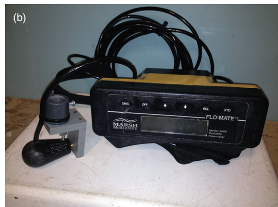
Figure 5.6 Current velocity can be measured using various meters: (a) a propeller design that counts revolutions of a spinning blade, (b) an electromagnetic meter that measures changes to the electromagnetic field around its bulb to estimate velocity. (Source: Darren Ryder.)
