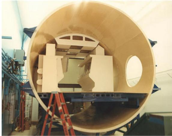
developed a full-scale mockup in which to portray and evaluate their design concepts. Figure 3.6a, b shows views of the TransHab mockup, built from traditional flat and rigid materials to convey the rigid structural endoskeleton (axle) of the TransHab Concept. The TransHab mockup was a landmark of TRL-2 concept formulation because it displayed credibly how the interior of this toroid could be made useful.
