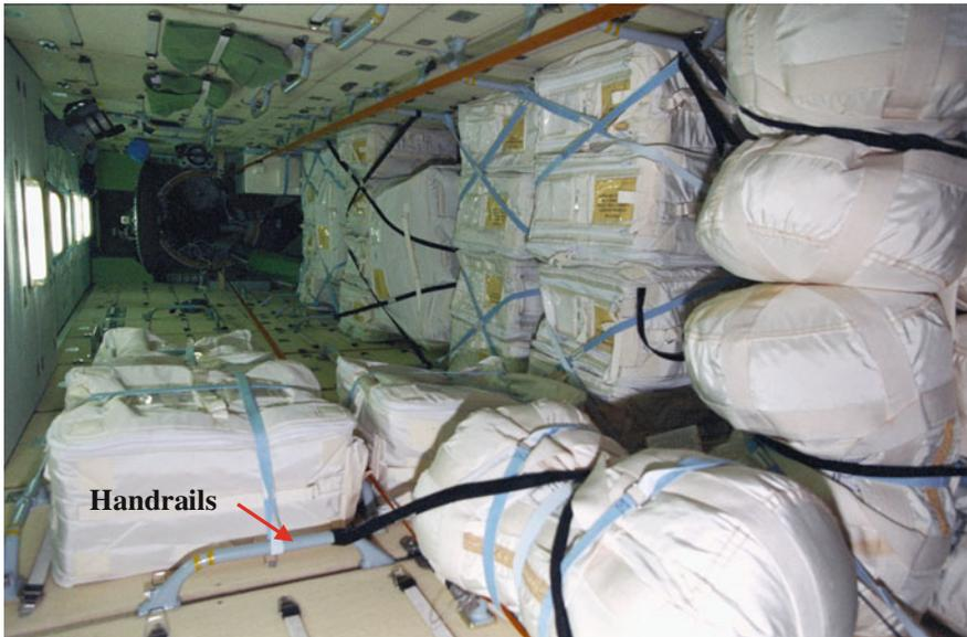
**Fig. 4.4** The interior of the module FGB/zarya, showing the handrails and stowage panels (1996). STS096-378-037 (NASA)
