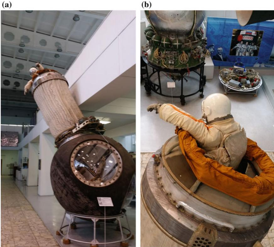
**Fig. 5.26** a and b an inflatable airlock of Voskhod-2 spacecraft functioned well but the entry hatch was too small
