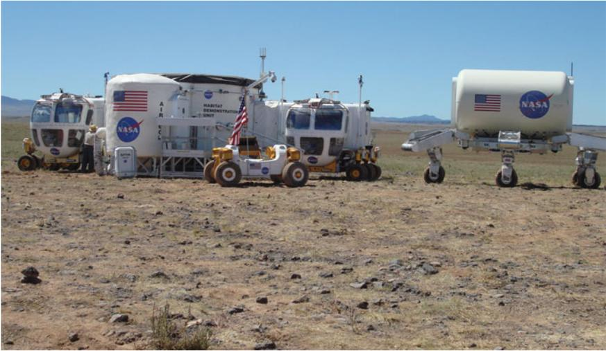
**Fig. 5.23** Two rover prototypes docked to the Habitat Demonstration Unit, next to the Athlete vehicle (NASA)
