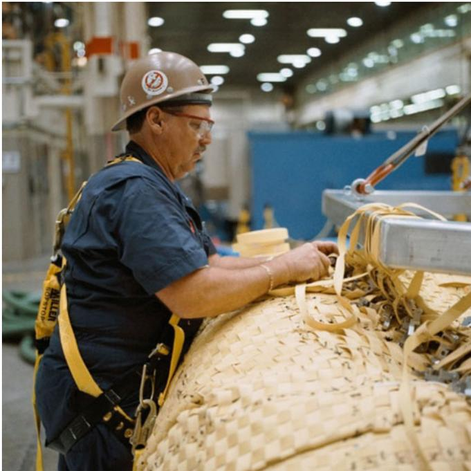
**Fig. 6.24** TransHab Full Scale Demonstration Unit Restraint Layer Assembly (NASA)
