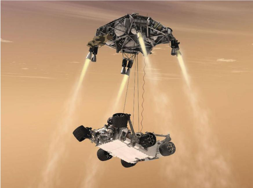
**Fig. 5.3** Having ejected the lower heat shield and the parachute, this image shows the sky crane lowering the rover onto the Martian surface (NASA/JPL-Caltech)
