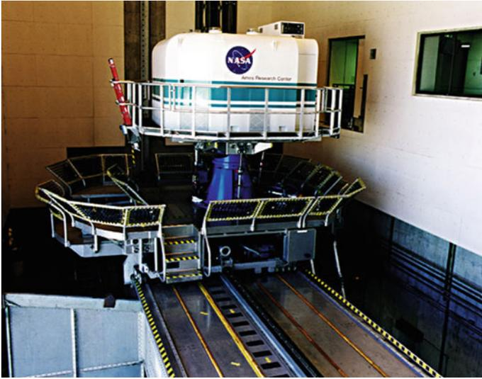
**Fig. 3.18** Vertical Motion Simulator, NASA Ames. The cab sits on a three-degree of freedom motion base that provides roll, pitch, and yaw. This motion base is on a bridge track with 12 m lateral motions. The bridge affords 24 m of vertical motion (NASA)
