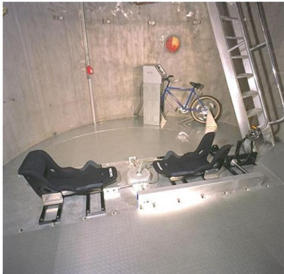
**Fig. 3.28** Lower level of the CERC with the Human Powered Centrifuge in operation (NASA)
