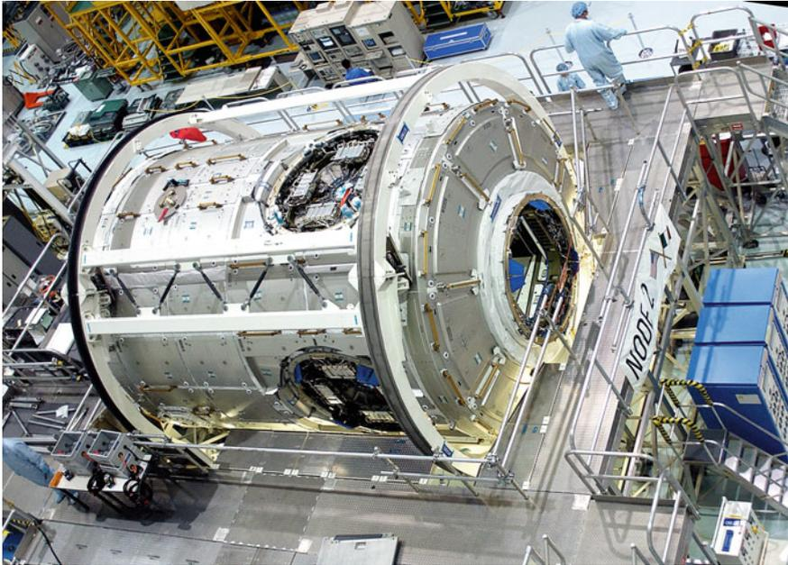
**Fig. 5.5** ISS Node 2 (Harmony) module under construction (NASA)
