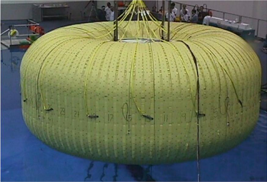
**Fig. 6.21** TransHab hydrostatic test #1 ~30 psid (NASA)
