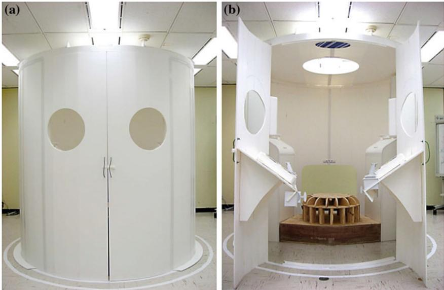
**Fig. 3.2** a Exterior view of the Altair Ascent Module Mockup, showing the pilot windows (Cohen 2006). b View of the Ascent Module interior with the engine head represented on the floor and the “EVA Hatch” behind it (Cohen 2006)
