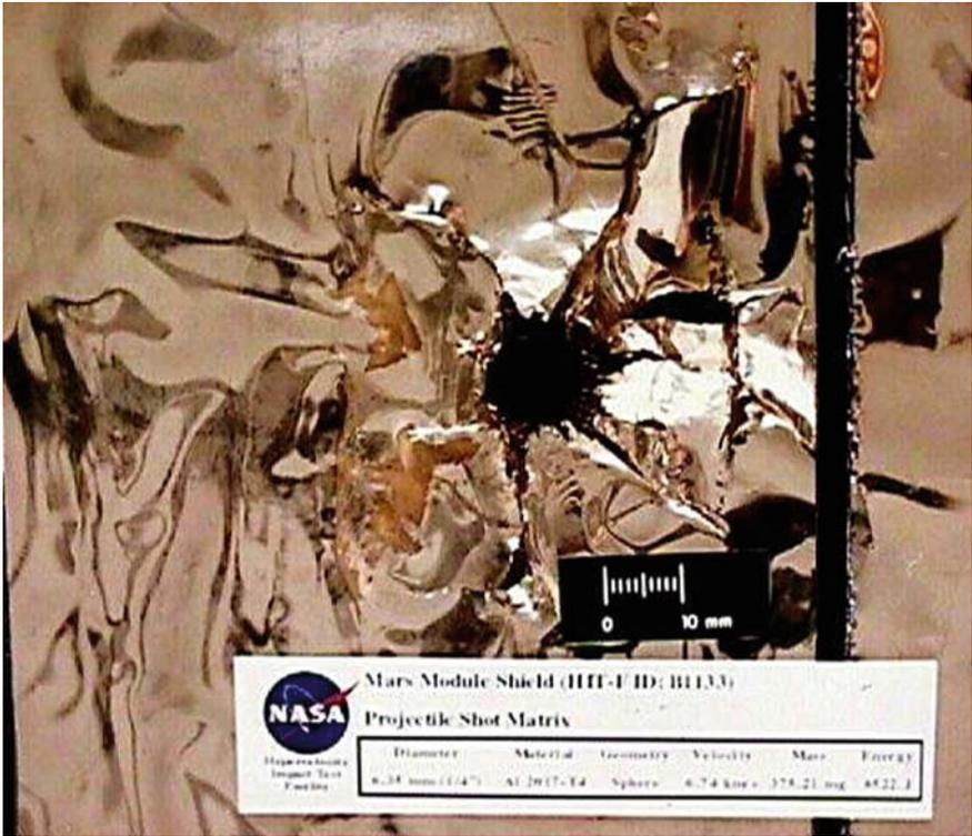
Fig. 6.16 TransHab shell MM/OD hypervelocity impact test (NASA)
