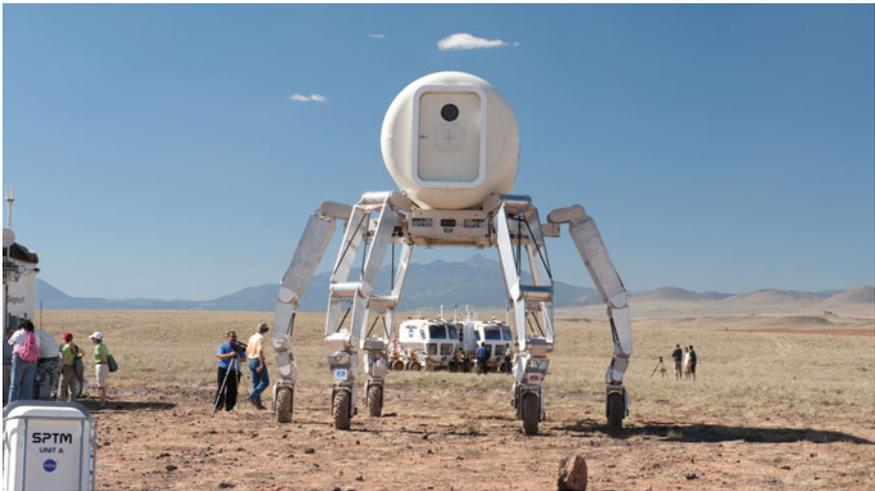
Fig. 5.22 Tri-ATHLETE with a Hab module on the top (NASA)
